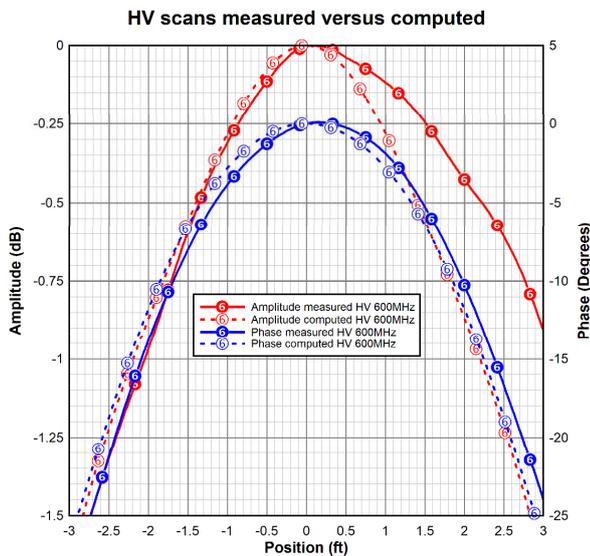
Figure 6. Computed and measured amplitude and phase at 600 MHz for range B.
