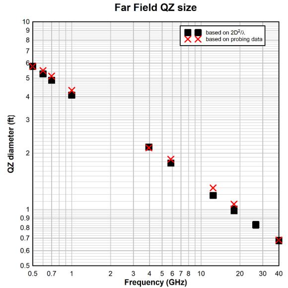
Figure 10. Computed and measured far field illuminated QZ for range B.
