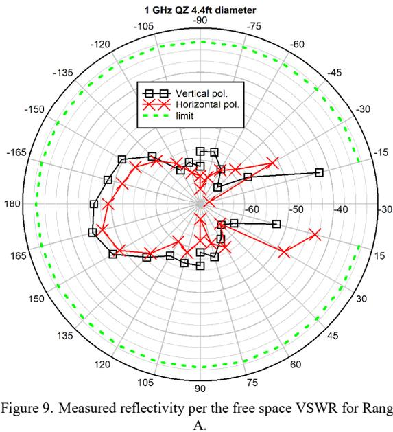
Figure 9. Measured reflectivity per the free space VSWR for Range A.
