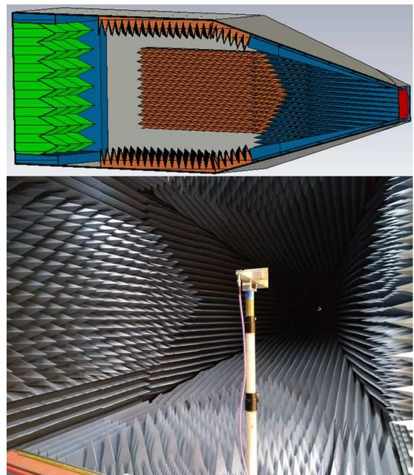
Figure 1. Range A shown above in the CST Suite model (some absorber and the conical feed hidden for clarity) and below a picture of the implemented range.
