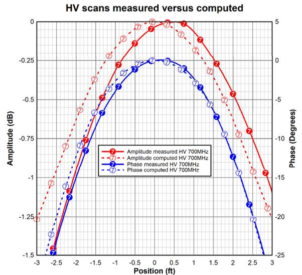
Figure 7. Computed and measured amplitude and phase at 700 MHz for range B.
