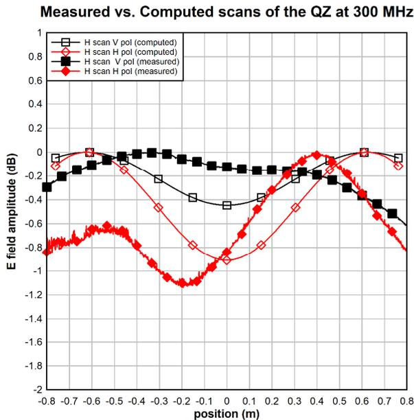
Figure 3. Measured and Computed scans for two orthogonal polarizations of the range antenna at 300 MHz.
