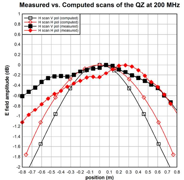
Figure 4. Measured and Computed scans for two orthogonal polarizations of the range antenna at 200 MHz.
