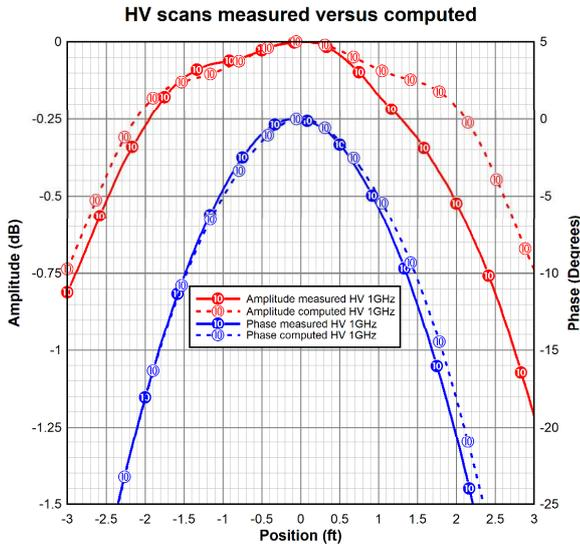
Figure 8. Computed and measured amplitude and phase at 1 GHz for range B.
