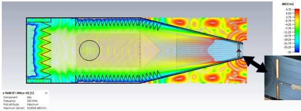
Figure 2. Model of the tapered range showing the dipole excitation, the inset picture shows the dipole used as a range antenna at the 100 to 300 MHz range. Because the conical feed section is not present the structure is “unshielded”
