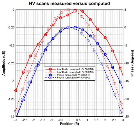
Figure 5. Computed and measured amplitude and phase at 500 MHz for range B.
