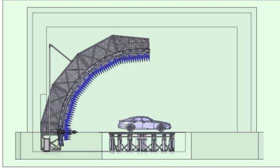
Figure 4. SNF Chamber for Automotive Measurements
