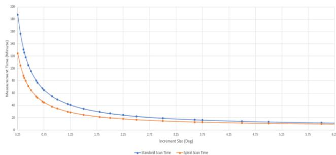
Figure 9. Measurement Time vs Increment Size
