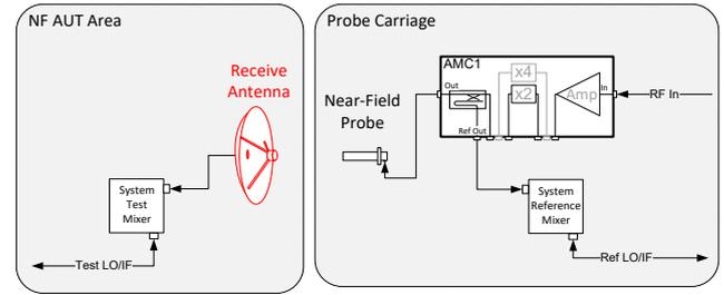
Figure 2. Reference diagram showing an RF signal being injected into the transceiver receive antenna.
