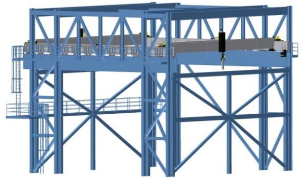
Figure 5: Dual-Bridge Horizontal Planar Near-Field Scanner [8]
