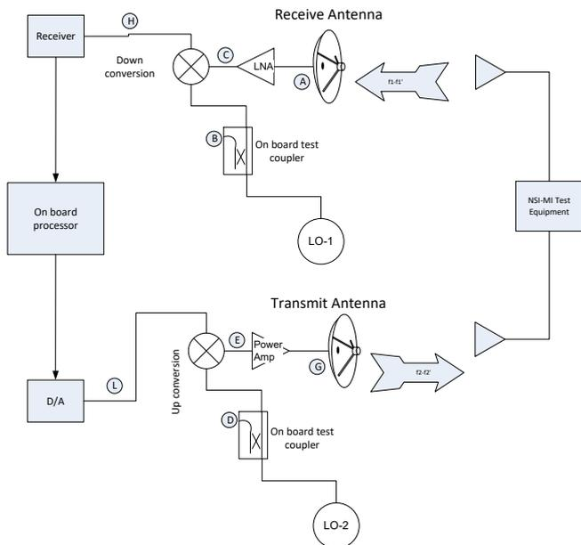
Figure 1. E2E Reference diagram showing transceiver architecture and test point references.
