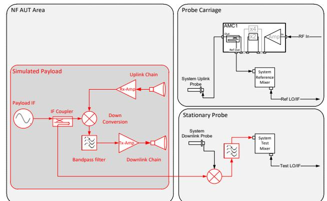
Figure 6: Simulated payload and modified RF test system with secondary mixer shown.
