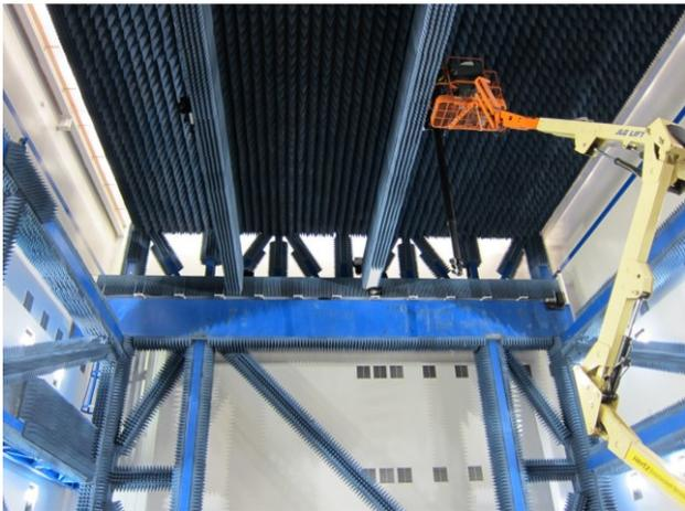
Figure 4: Dual-Bridge Horizontal Planar Near-Field Scanner [8]
