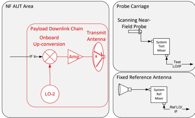
Figure 3. Modified RF test system with fixed reference antenna.
