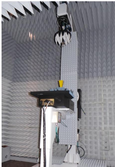
**Figure 3: A swing arm ( $\theta/\phi$ ) spherical near-field antenna test system used for mm-wave applications.**
