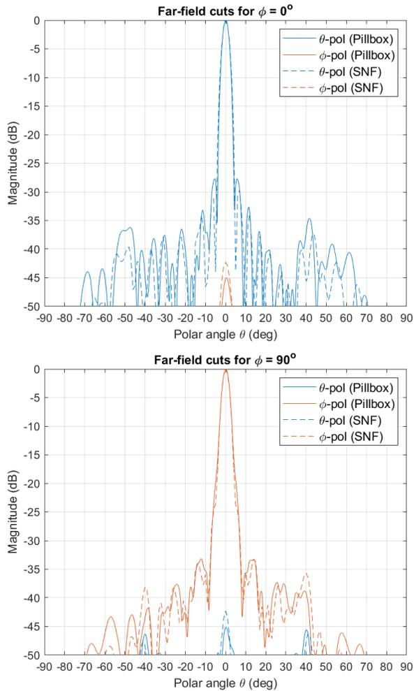
**Figure 7: Orthogonal principal plane radiation pattern cuts shown for the AUT. FlexForm result is depicted as the solid lines and Spherical Near-Field as dashed lines.**
