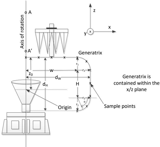
**Figure 2: The generatrix parameters and coordinate system defined.**
