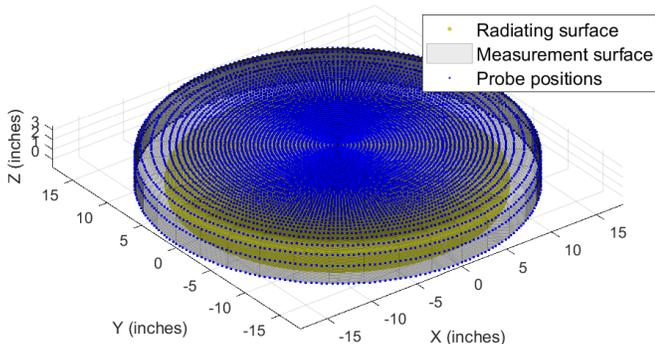
**Figure 4: Graphical representation of the field sample locations (blue dots) where near-field samples are acquired on the capped cylinder.**
