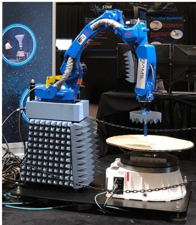
**Figure 1:** The six-axis robotic arm, rotation stage and AUT are shown. In this instance the AUT is a slotted waveguide array and the near-field probe is a linearly polarized open-ended waveguide probe.
