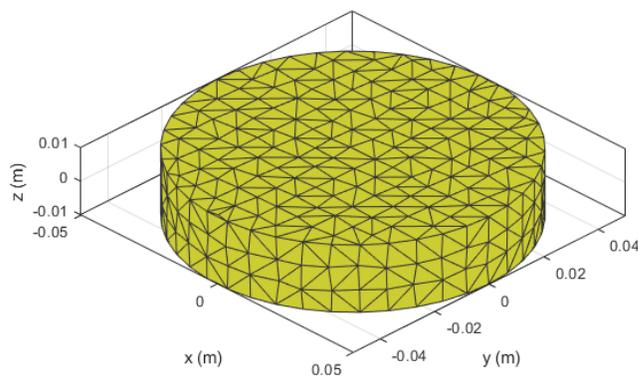
**Figure 6: Example discretized AUT bounding surface.**
