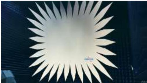
Figure 4. A Compact range designed to operate down to 700MHz for base station antenna testing
