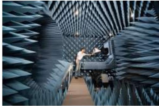
Figure 5. A combined SNF and Taper range. The AUT positioner is being shown from the near field probe stand. To the left the conical taper section is shown. The ranges are perpendicular to each other sharing the AUT positioner
