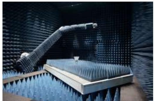
Fig. 3. A large in-door near field gantry for on-vehicle antenna measurements. A Standard Gain Horn (SGH) is being measured.
