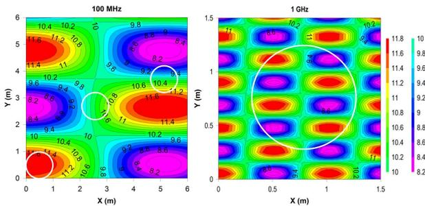
Figure 3. Simulated interference from reflections at 100 MHz and 1 GHz for a 1m Diameter QZ.
