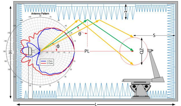
Figure 1. An Anechoic chamber geometry showing the different parameters. The width W is not shown but it will be analogous to the height H.
