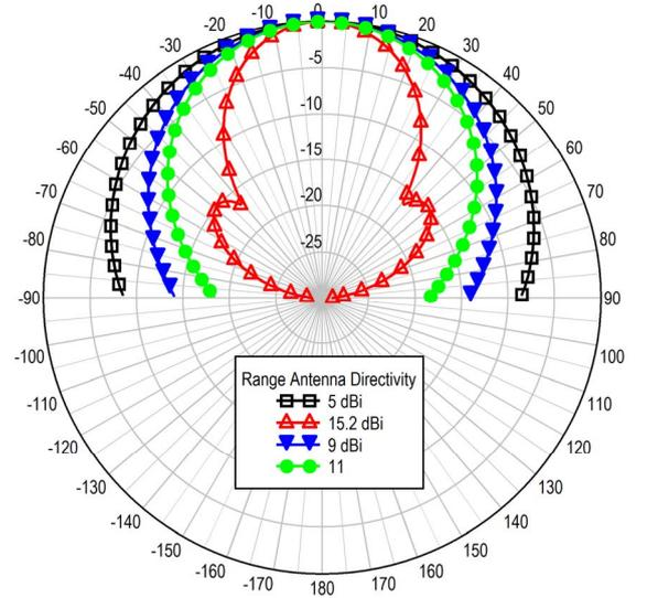
Figure 2. Approximated patterns for the range antennas for range 1.
