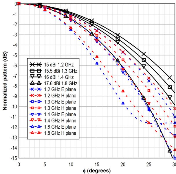
Figure 4. Patterns for a Seavey SGA-10 SGH used as source antenna compared to the approximated patterns used in the analysis.
