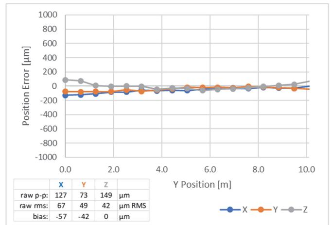
Figure 3. Sampled XYZ probe position errors *after* monument update corrections.
