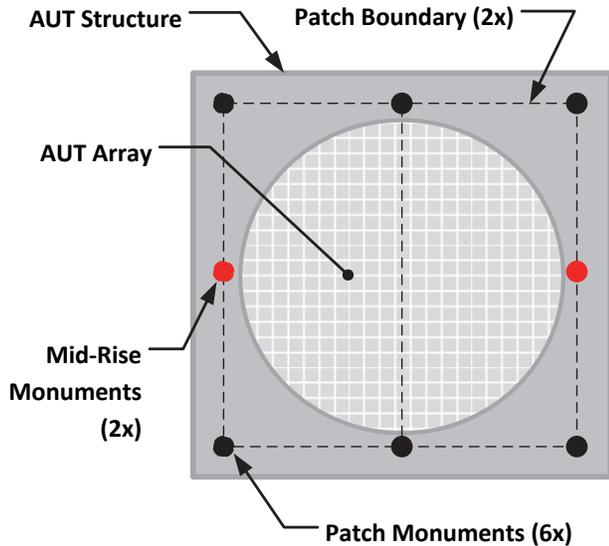
Figure 4. An eight-monument set mounted to the AUT structure, configured into two patches with two mid-rise monuments.
