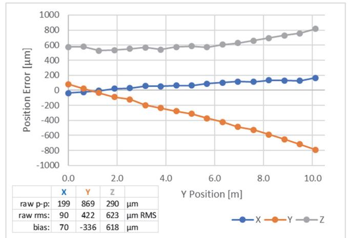
Figure 2. Sampled XYZ probe position errors *before* monument update corrections.
