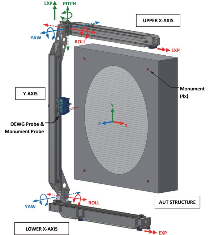
Figure 1. Vertical PNF scanner design with additional DOFs to account for thermal effects. AUT is shown with four perimeter monuments.
