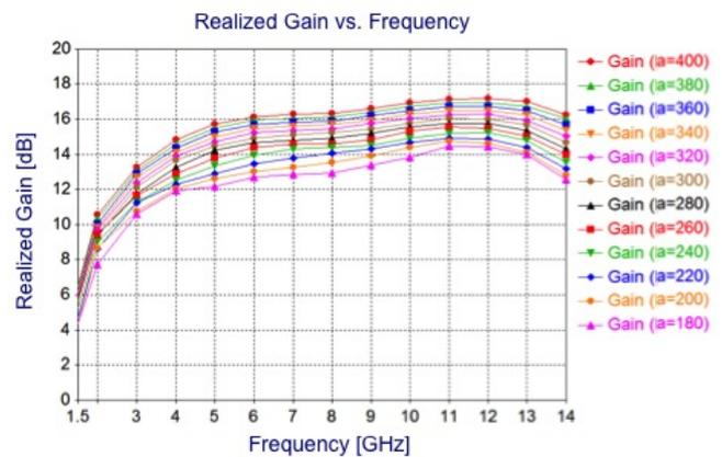
Fig. 2. Gain as a function of frequency for OQRH Type-A profile for different values of scaling parameter (arbitrary units)
