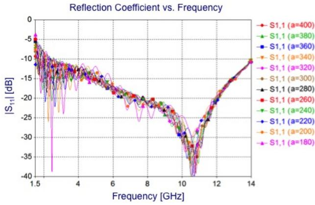
Fig. 3. Input reflection coefficient as a function of frequency for OQRH Type-A profile for different values of scaling parameter (arbitrary units)
