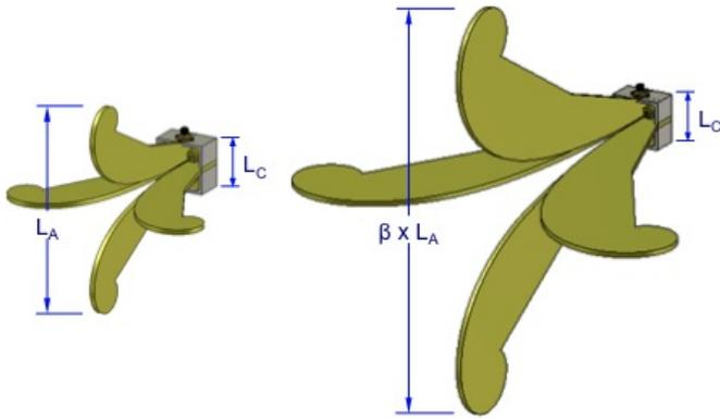
Fig. 4. Scaling of a QQRH Type-B while maintaining the launching section invariant.
