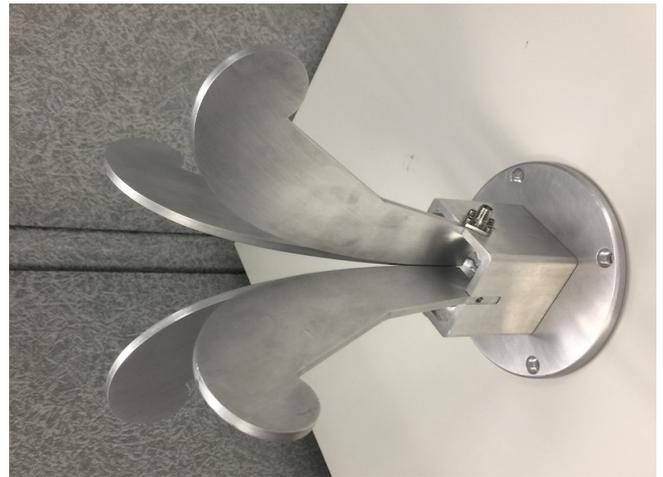
Fig. 7. Manufactured OQRH Type-B design ( $CC=72$ ).
