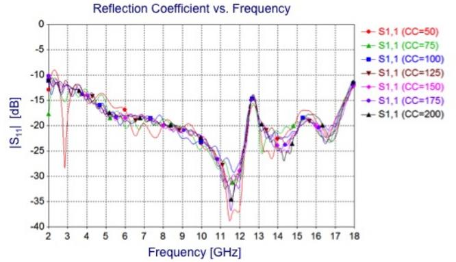
Fig. 6. Calculated input reflection coefficient as a function of frequency for OQRH Type-B profile for different values of scaling parameter (arbitrary units)
