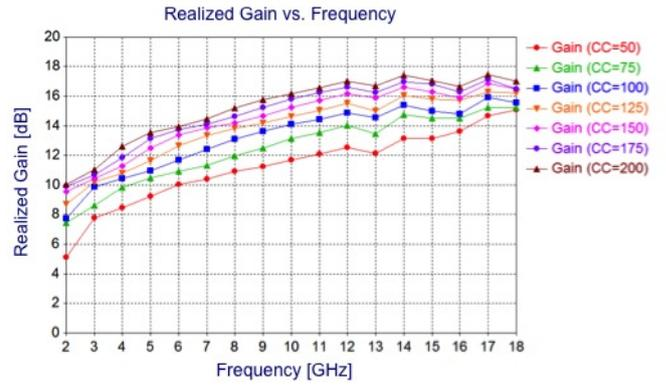
Fig. 5. Gain as a function of frequency for OQRH Type-B profile for different values of scaling parameter (arbitrary units)
