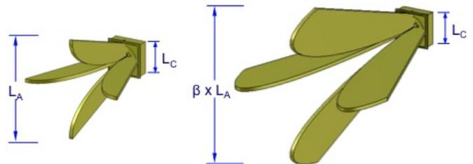
Fig. 1. Scaling of a Open Boundary QRH (OQRH) Type-A profile while maintaining the launching section invariant.
