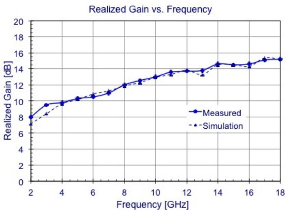
Fig. 9. Comparison between measured and simulated realized gain as a function of frequency for manufactured OQRH Type-B profile. The dashed line corresponds to the simulated response.
