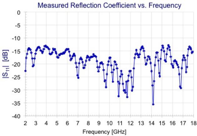
Fig. 8. Measured Input reflection coefficient as a function of frequency for manufactured OQRH Type-B profile.
