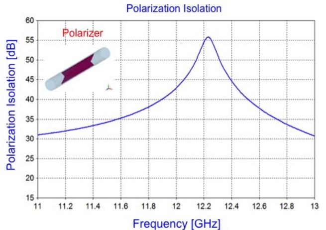
Fig. 2.  $90^\circ$  phase shifter design: Calculated polarization isolation of the Rexolite polarizer plated in CST
