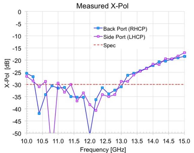
Fig. 6. Measured circularly polarized compact range feed cross-polarization response.
