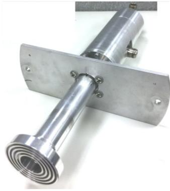
Fig. 3. Fabricated dual port, circularly polarization compact range feed from 10 GHz to 15 GHz.
