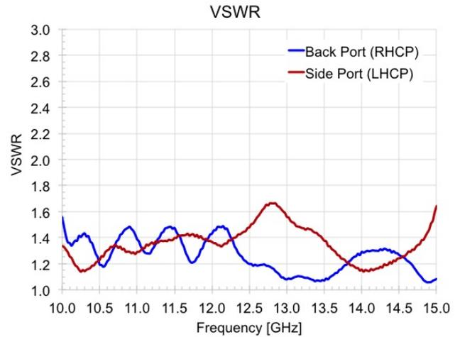
Fig. 5. Measured compact range feed input VSWR.
