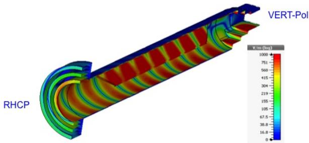
Fig. 1. Conversion from vertical linear polarization to RHCP fields when they pass through the waveguide polarizer section to the aperture of the feed in CST simulation at 12 GHz.
