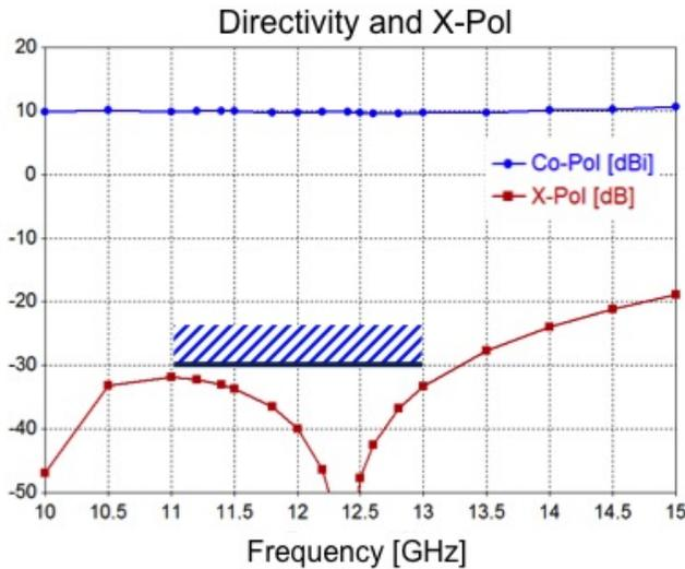
Fig. 4. Calculated directivity (blue circles) and cross-polarization (red squares) of the circularly polarized compact range feed design, indicating the frequency band of interest for the cross-polarization response.
