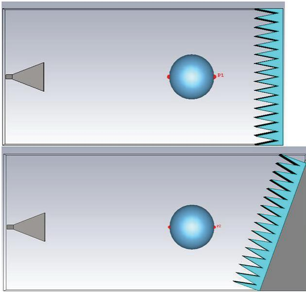
Figure 4. The two numerical experiments. The top is a SGH illuminating a standard wall of 72-inch pyramids, the bottom is the same SGH illuminating a tilted wall treated with the same 72-inch pyramids.
