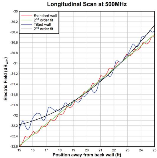
Figure 6. Longitudinal scans for the standard wall and the tilted wall. A second order fit has been added for analysis of the ripple.
