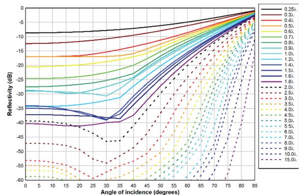
Figure 2. Bi-static reflectivity of pyramidal absorber of different thickness as reported in [4]
