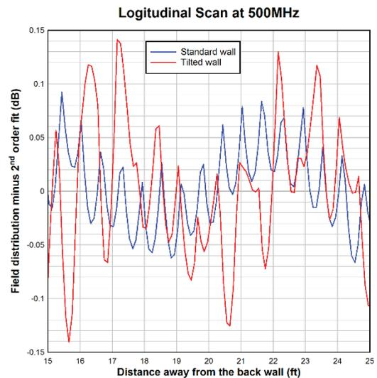
Figure 7. Distribution of the field in the QZ minus the 2<sup>nd</sup> order fit for the two cases being analyzed.
