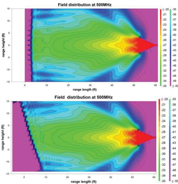
Figure 5. Field Distribution at 500 MHz for both the standard wall and the tilted wall.
