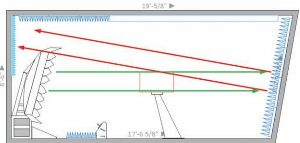
Figure 1. A RCS compact range with a 10-degree tilted wall.
