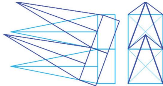
Figure 3. Side and front view of 72-inch regular pyramids with and without a 20-degree tilt.
