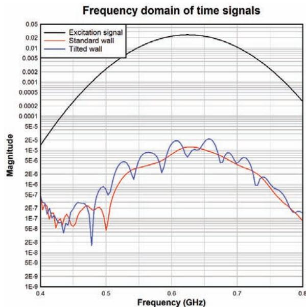
Figure 9. Frequency spectrum of the excitation and the signals reflected from the back wall at the excitation port.
