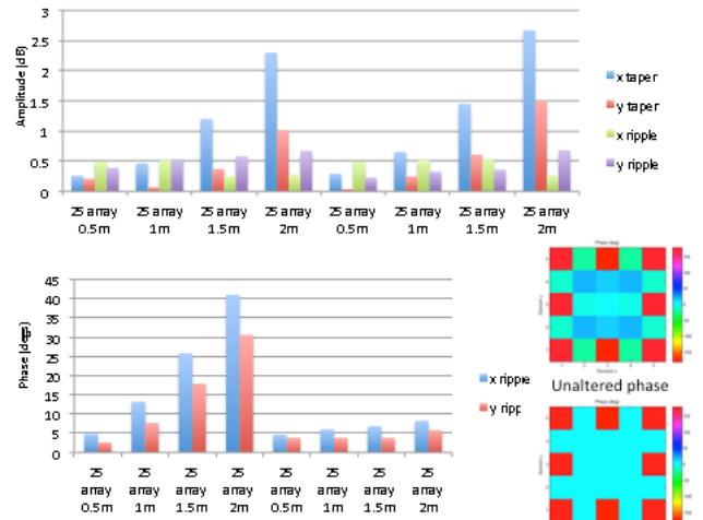
Fig 12. Summary of results for the symmetrical back-projected target function used in figure 10, left hand side= array excitation phase unaltered; right hand side= array excitation phase quantised to  $0^\circ$  and  $180^\circ$ . Inset figure shows array excitation phase unaltered (top) and quantised (bottom).
