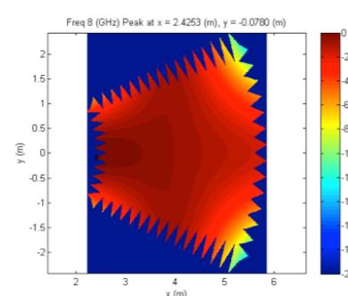
Fig 4 Simulated CATR field for 9 element array feed with serrated reflector edge.
