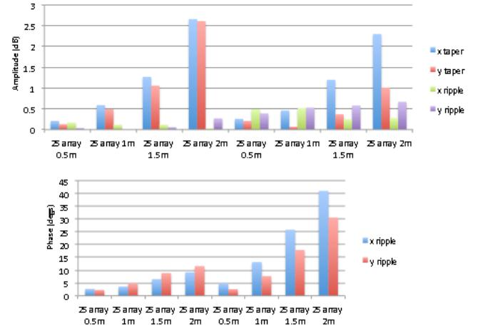
Fig 11 , Summary of results for the symmetrical back-projected target function used in figure 10 – right hand side, compared to the Gaussian target pattern of Fig.8 – left hand side. Amplitude taper and ripple (top) and Phase ripple (bottom).
