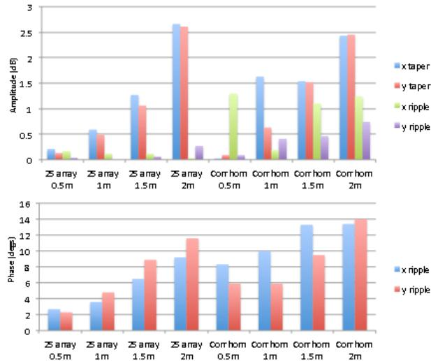
Fig 9 Summary of results for the shaped target function used in figure 8, compared to the corrugated horn feed. Amplitude taper and ripple (top) and Phase ripple (bottom).
