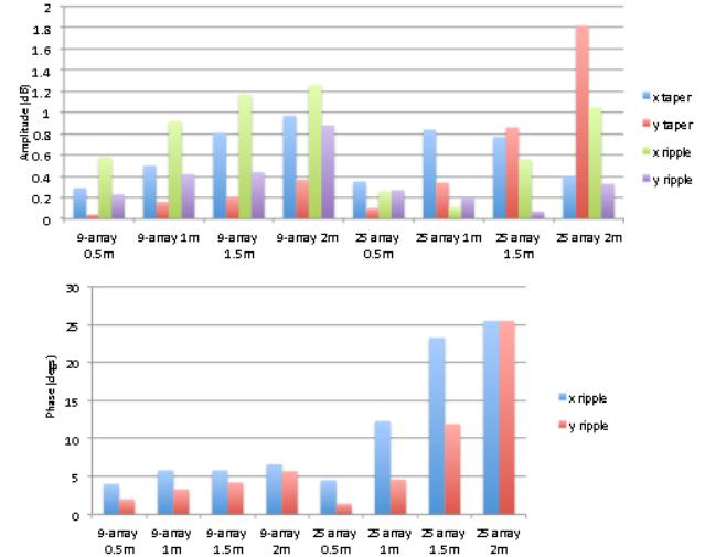
Fig 7. As fig 6 but with 25 element array feed using target function accounting for  $1/r$  amplitude taper and increased iteration count (16,000). Amplitude taper and ripple (top) and Phase ripple (bottom).
