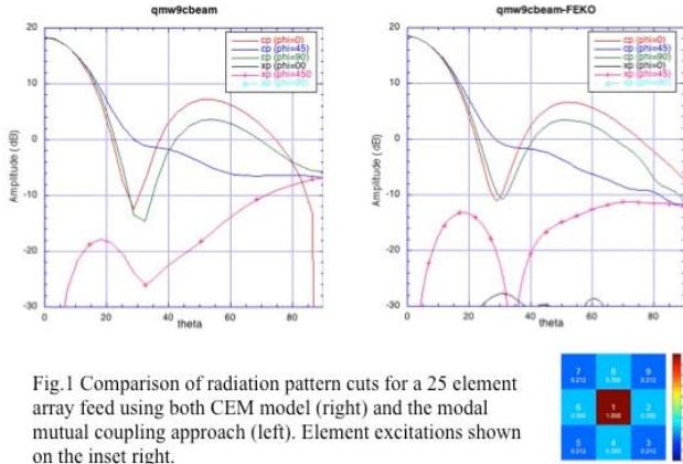
Fig.1 Comparison of radiation pattern cuts for a 25 element array feed using both CEM model (right) and the modal mutual coupling approach (left). Element excitations shown on the inset right.
