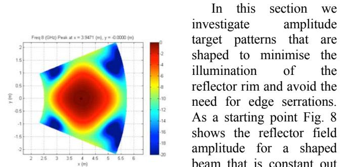
Fig. 8 Reflector amplitude for target function that is constant out to  $7^\circ$  and then Gaussian down to -20dB at reflector edge.
