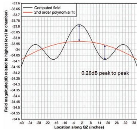
Fig. 7. Transverse Scan of the QZ along the Vertical Axis
