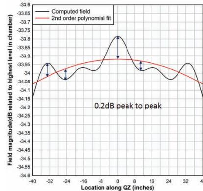
Fig. 8. Transverse Scan of the QZ along the Horizontal Axis
