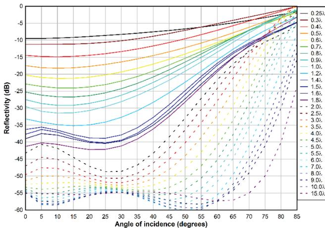
Fig. 1. Plots of the Reflectivity of RF Absorber from Equation (1)
