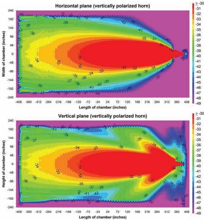
Fig. 5. Field distribution at 700 MHz in the large far field range in the horizontal and the vertical planes. Note the SQZ pattern of the source antenna.
