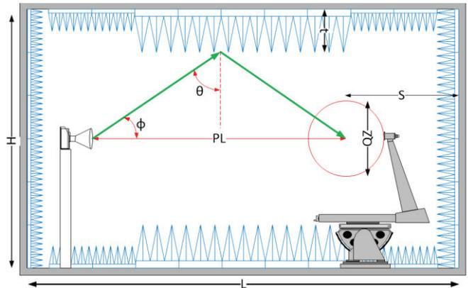
Fig. 2. Geometry of a Rectangular Anechoic Range
