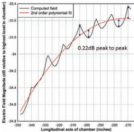
Fig. 6. Longitudinal Scan of the QZ for the Large Far-Field Range at 700 MHz
