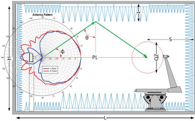
Fig. 3. A pattern of the source antenna superimposed on the chamber diagram showing that the level of energy emitted towards the specular point is lower than the level of the direct ray along the path length PL.
