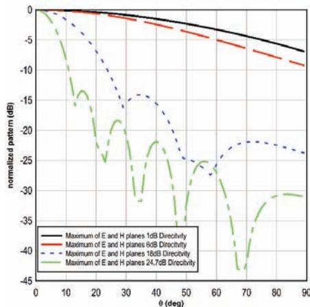
Fig. 9. Assumed Patterns used for the Analysis of the Measured Chamber
