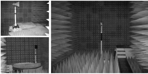
Fig. 11. Views of the anechoic chamber being analyzed.
