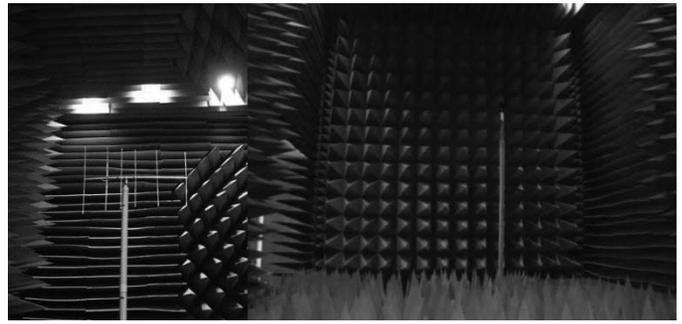
Fig. 10. Two pictures of the testing of the chamber. On the left, a large Yagi is used to scan the QZ at 100 MHz seen from the side wall of the chamber. On the right, a horn is used to scan at 12 GHz as seen for the source wall.
