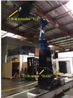
Figure 11. Positions of the laser tracker targets on the MR base and TCP to measure cross range movement while the MR is moving.
