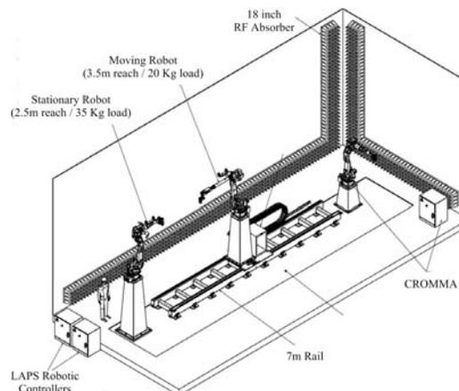
Figure 1. The Large Antenna Positioning System and CROMMA co-located in the NIST Advanced Communications Metrology Laboratory.
