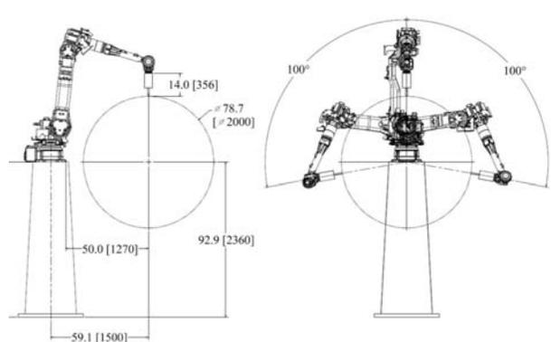
Figure 5. Stationary Robot typical spherical scan plane geometry in inches [mm].
