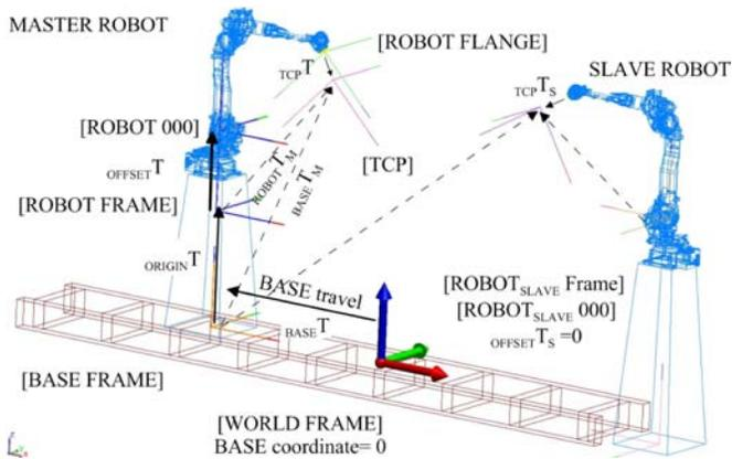
Figure 2. Extrinsic frames, e.g. [BASE], and the 6D solid-line transforms ( $BASE T$ ,  $ORIGIN T$ ,  $OFFSET T$ ,  $TCP T$ ) between them, determined during calibration of a robot's kinematic model. This allows more accurate knowledge of tool location (dashed lines:  $ROBOT T_M$ ,  $BASE T_M$ ) using only the robot controller. Similar measurements are made for the SLAVE/stationary robot (SR).
