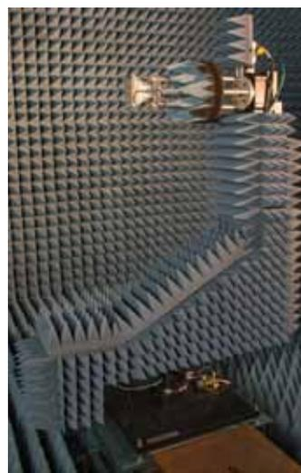
Figure 2: Spherical Near-Field Scanner
