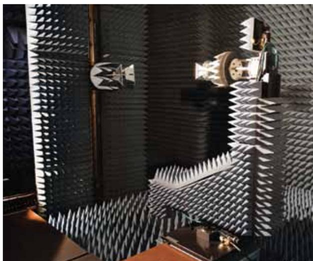
Figure 1: Anechoic Chamber
