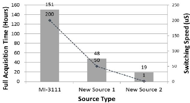
Figure 3. Effect of Signal Source Switching Speed
