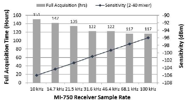
Figure 1. Receiver Sample Rate Tradeoffs
