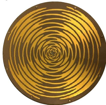
Figure 1. Photo of dual-port sinuous feed antenna
