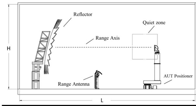
Fig. 1. Compact range geometry (side view)
