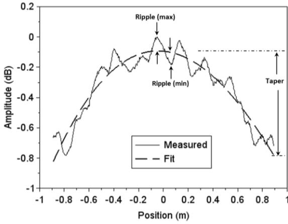
Fig. 2 Field probe amplitude Ka-band H-pol H-cut
