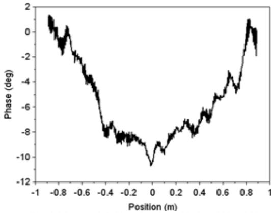
Fig. 3 Measured field probe phase Ka-band H-pol H-cut
