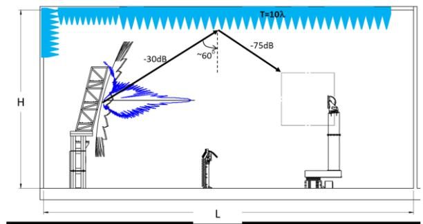
Fig. 6. Bistatic scattering from microwave absorber
