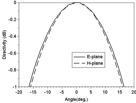
Fig. 8 E&H plane simulated range antenna pattern, Ka-band
