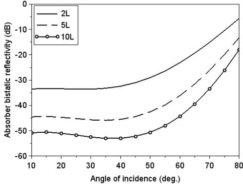
Fig. 7. Bistatic reflectivity for pyramidal absorbers of different electrical thicknesses ( $L=\lambda$ )
