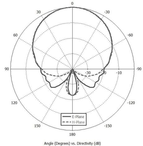
Fig. 4 Range antenna radiation patterns E and H planes
