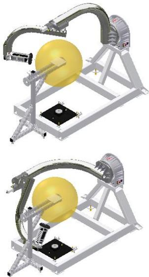
Figure 3. Two distinct probe positions are depicted. Top:  $\theta = 135^\circ$  &  $\phi = 0^\circ$ . Bottom:  $\theta = 135^\circ$  &  $\phi = -90^\circ = 270^\circ$ .
