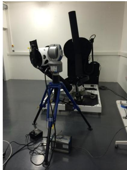
Figure 4. Structural measurement using a laser tracker. Note that only a portion of the full spherical surface can be evaluated.
