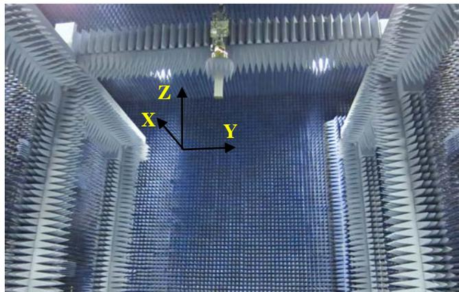
Figure 1. MI-815-26x20 8m x 6m HPNF scanner
