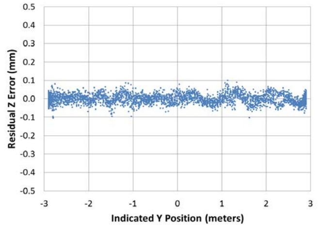
Figure 8. Spinning-laser residual for Y scans
