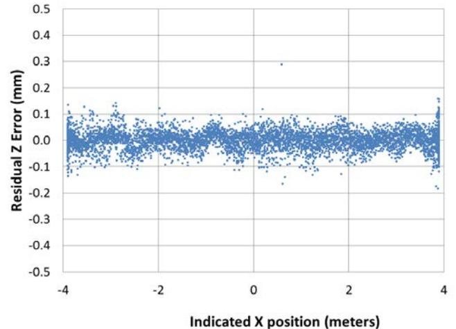
Figure 9. Spinning-laser residual for X scans
