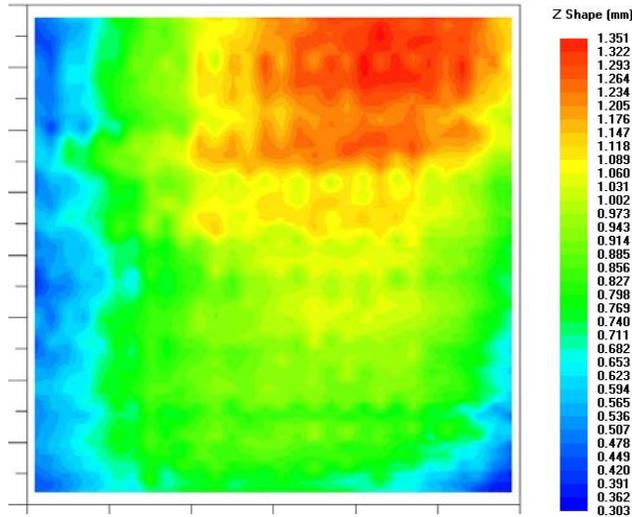
Figure 10. Planarity corrected by spinning laser
