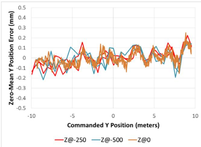
Figure 7. Tracking-laser residual Y error
