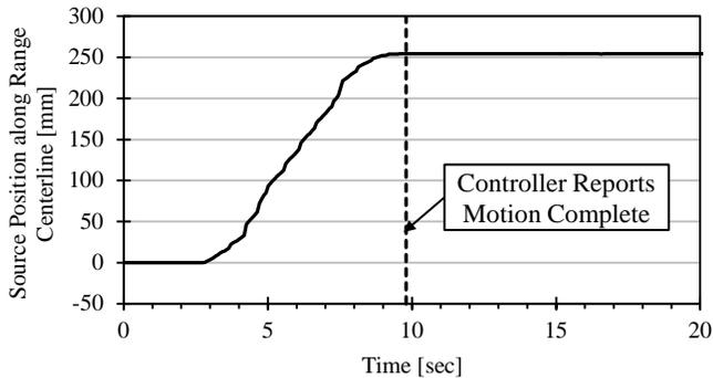
Figure 5. Measured Source Motion as Floorslide Traverses along Range Centerline
