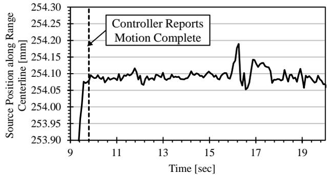
Figure 6. Raw Measured Source Motion after Controller indicates Motion is Complete
