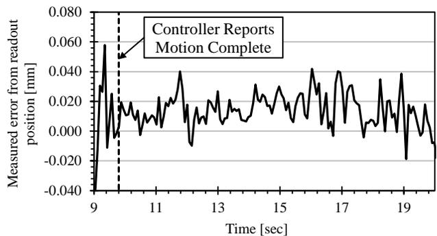
Figure 7. Measured Position Error from Controller Readout Position
