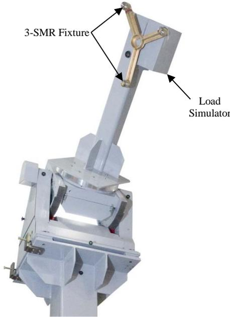
Figure 4. Test Article Simulator with SMR Fixture
