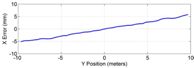
Fig. 3. Uncorrected  $\Delta X(Y)$  During Calibration
