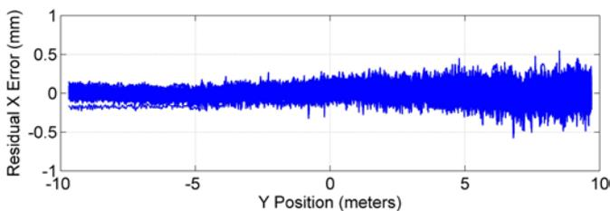
Fig. 5. Residual  $\Delta X(Y)$  During Acquisition (0.06 mm RMS)
