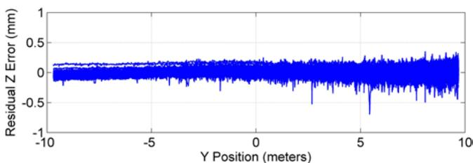
Fig. 4. Residual  $\Delta Z(Y)$  During Acquisition (0.05 mm RMS)
