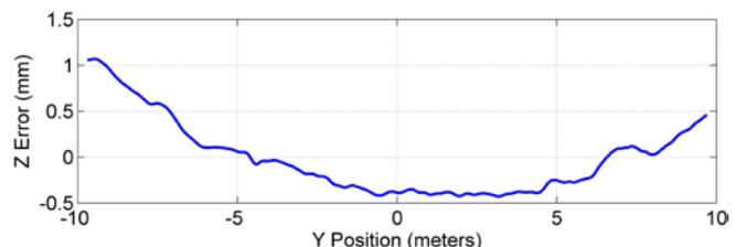
Fig. 2. Uncorrected  $\Delta Z(Y)$  During Calibration
