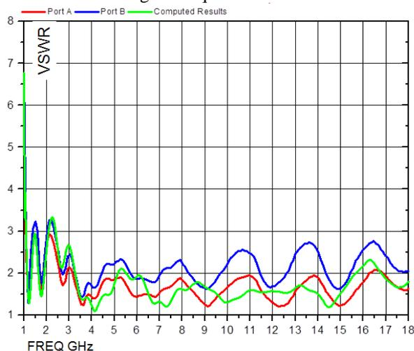
Fig. 6. The measured and computed VSWR for the quad ridge horn introduced in [2] showing the higher differences at higher frequencies.
