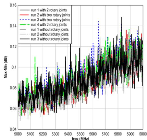
Fig. 5. Verification of the measurement system in the frequency band.
