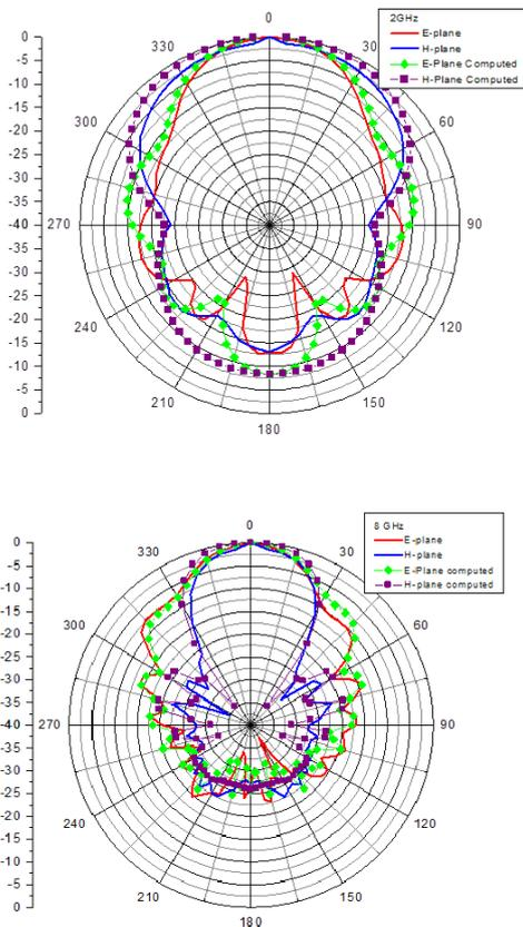
Fig. 7. The measured and computed radiation patterns at 2GHz (top) and 8GHz (bottom) for the antenna introduced in [2].
