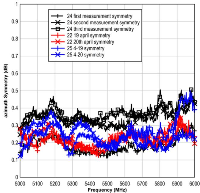
Fig. 3. Measured results for the prototypes. Three separate units labeled 24, 25 and 22, measured different times. The azimuth symmetry or variation on the pattern around the dipole axis is larger than 0.2 dB.
