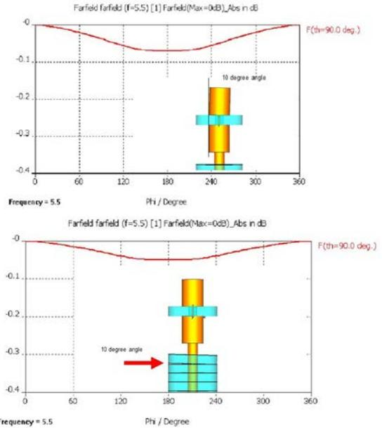
Fig. 4. Variation of the radiation in azimuth for one case with the top element bent by 10 degrees and a second case with the first choke section bent by 10 degrees.
