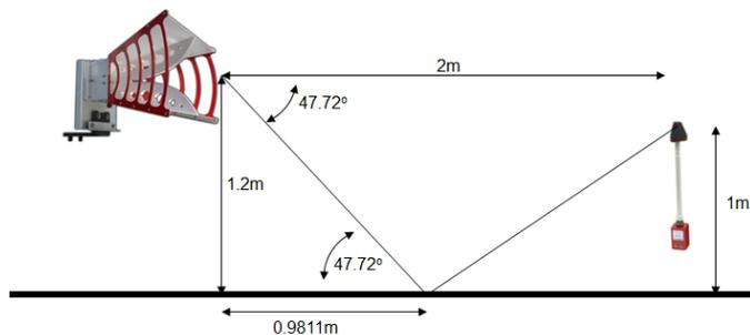
Fig. 9. The geometry of the test per the ISO 11451-2 standard. The reflected ray is about 9dB lower than the direct ray to the broadband field probe.
