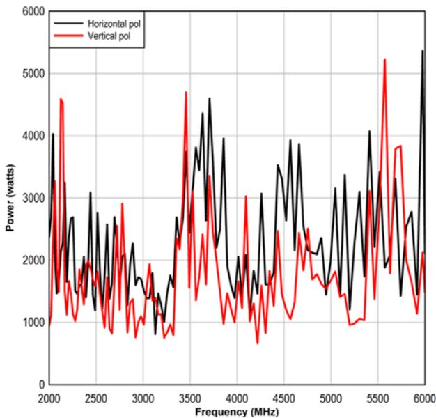
Fig. 8. Measured power required at the antenna input to generate 100V/m at 2m distance and 1m over a metal ground plane as required by ISO 11451-2 for automotive testing.
