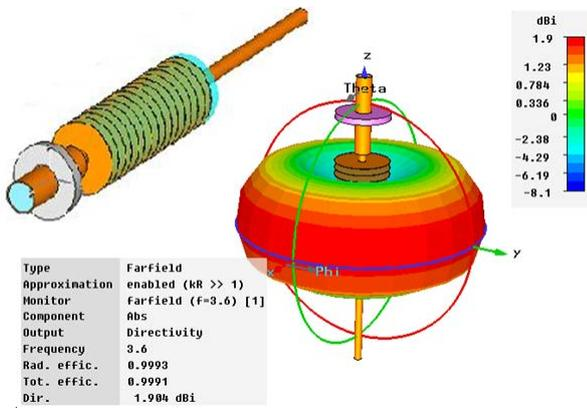
Fig. 2. Pattern results for 3.6 GHz version of the sleeve dipole . The dipole model is shown on the left. The round features along the feed cable are  $\frac{1}{4}$  wavelength chokes.
