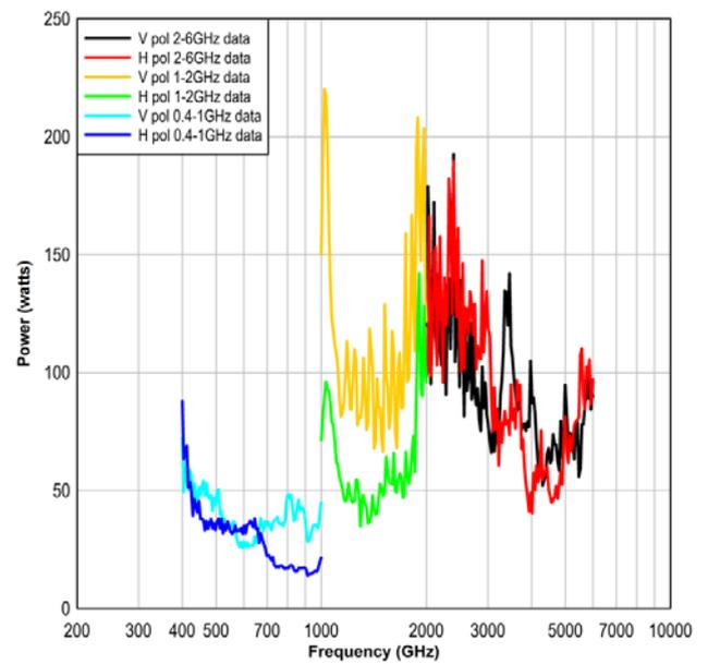
Fig. 10. Data measured per the ISO 11452-2 at different bands showing a large discontinuity at 1GHz.. Amplifiers and couplers are switched at 1, and 2GHz.
