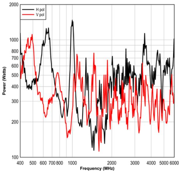
Fig.11. Measure data for the ISO 11451-2 showing a small transition at 1 GHz and 2 GHz. The data was taken after the proper coupling factor files were used for the power measurement.
