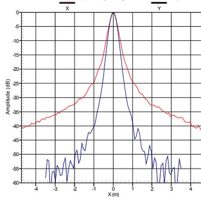
Fig. 1. Near-field X and Y amplitude cuts showing scan plane energy distribution for a WR650 SGH.
