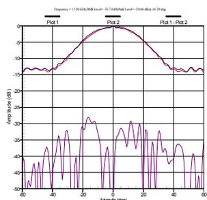
Fig. 7. Room scattering comparison Autz =  $Z_0$  vs  $Z_0 + \lambda/4$ . -35.7 dB RMS level MARS: OFF (includes truncation and leakage errors).
