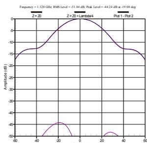
Fig. 8. Room scattering comparison Autz =  $Z_0$  vs  $Z_0 + \lambda/4$ . -51.8 dB RMS level MARS: ON (removes truncation and leakage errors).
