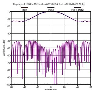
Fig. 5. Truncation level -46.3 dB without MARS (MARS: OFF).
