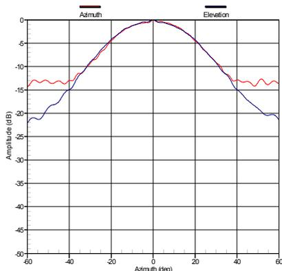
Fig. 2. Principal polarization Azimuth and Elevation cardinal cuts showing effects of scan plane truncation, finite dynamic range, and RF leakage.
