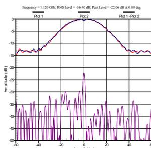
Fig. 9. Mutual coupling comparison ProbeZ =  $Z_0$  vs  $Z_0 + \lambda/4$ . -36.4 dB RMS level MARS: OFF (includes truncation and leakage errors).
