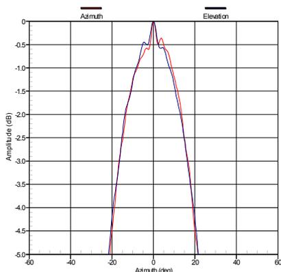
Fig. 3. Leakage effects on large planar scan can be seen to correspond to a very sharp sinc ( $\sin x/x$ ) function centred at 0° in Azimuth and Elevation. Here, axes of the plot have been adjusted to emphasise this effect.
