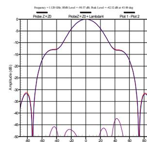
Fig. 10. Mutual coupling comparison ProbeZ =  $Z_0$  vs  $Z_0 + \lambda/4$ . -50.4 dB RMS level MARS: ON (removes truncation and leakage errors).
