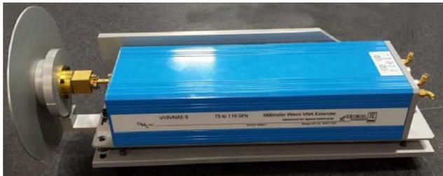
Figure 14. OML module with manually operated waveguide rotary joint.
