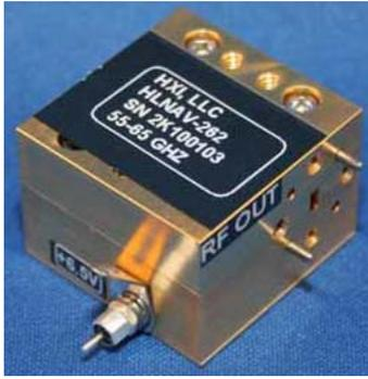
Figure 8. Example of Low-Noise Amplifier
