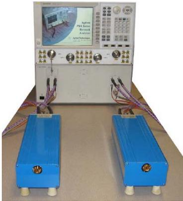
Figure 3. PNA with mm head controller and OML modules
