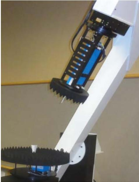
Figure 9. NSI-700S-85 Theta-over-Phi Swing Arm Spherical Near-Field Antenna Test System
