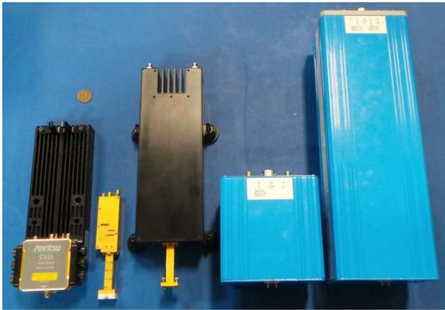
Figure 13. From left: Anritsu, VDI Micro, VDI Mini, OML VNA2-T and OML VNA2-S modules
