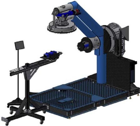
Figure 11. NSI-700S-86 Dual Swing Arm Spherical Near-Field Scanner for On-Chip mm-Wave Testing
