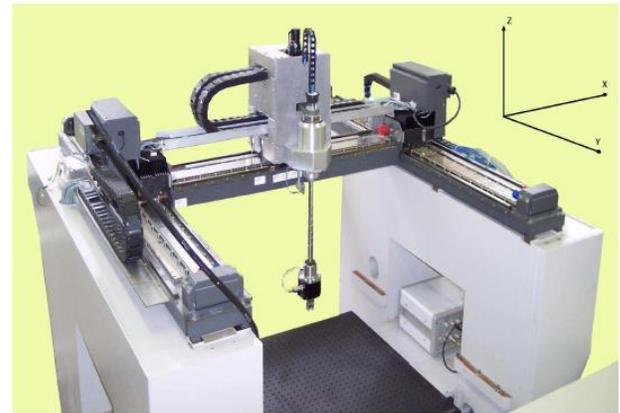
**Figure 9. Gantry XYZ pick-and-place positioner studied for the capabilities of gain scheduling<sup>[15]</sup>**
