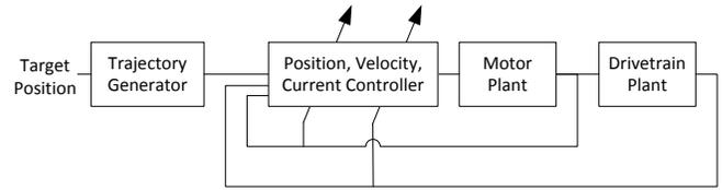
**Figure 8. Block diagram for state-based gain scheduling of a traditional positioner feedback loop**
