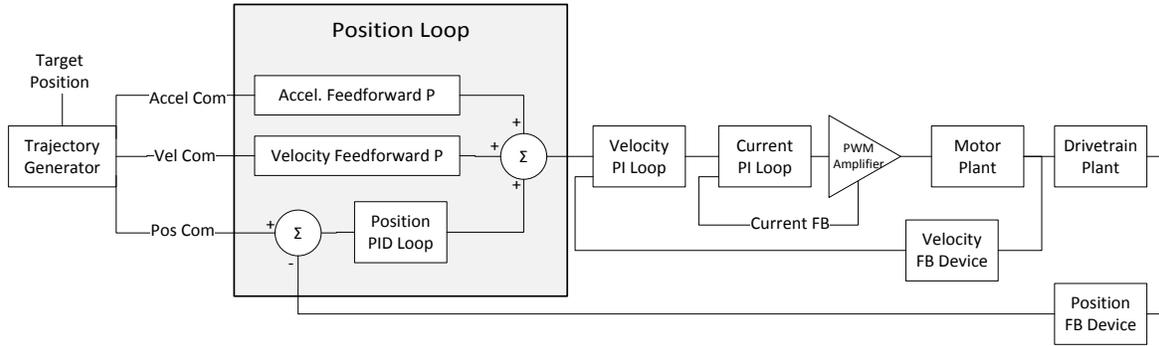
**Figure 2. Block diagram of advanced linear trajectory feedforward control in the MI-710C Position Controller**
