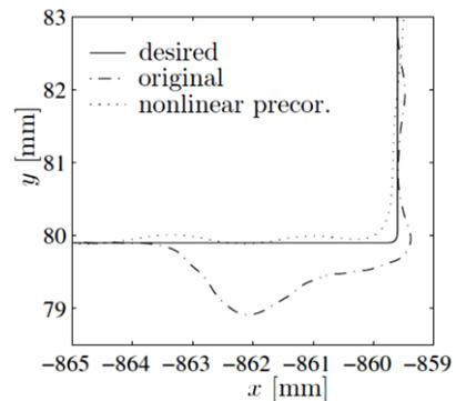
**Figure 7. Impact of a model-based feedforward controller compensating for friction and rigid-body dynamics in a Siemens manutec-r15 robot during a 2-axis traverse<sup>[13]</sup>**
