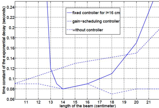
**Figure 10. Gain scheduling of PID parameters of the x-axis for a gantry XYZ positioner based on the overhang length of the z-axis beam shows large improvements in position settling time over fixed gains<sup>[15]</sup>**
