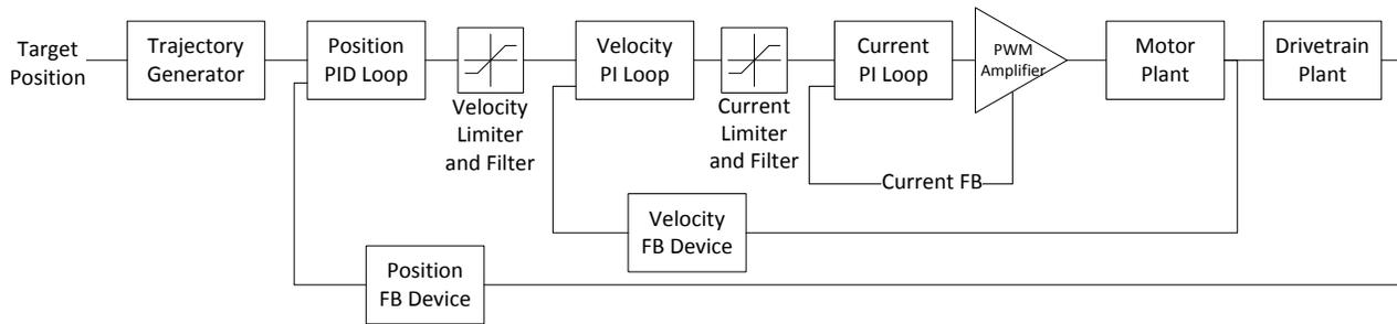
**Figure 1. Block diagram of typical positioner control system including linear current, velocity, and position feedback controllers**
