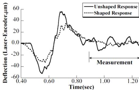
**Figure 5. Input shaping results show a significant reduction in unwanted dynamic excitation in a Coordinate Measuring Machine<sup>[8]</sup>**
