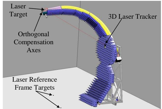
**Figure 3. Gantry measurement positioner with conceptual 3D closed-loop error compensation**
