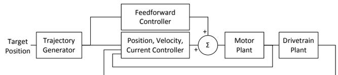
**Figure 6. Block diagram for model-based feedforward control**
