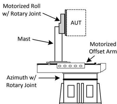
Figure 1 Roll over Azimuth Positioner Evaluated
