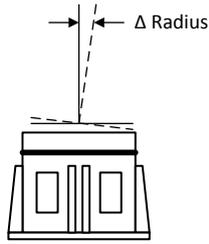
Figure 2 Radius Error due to Azimuth Axis Wobble
