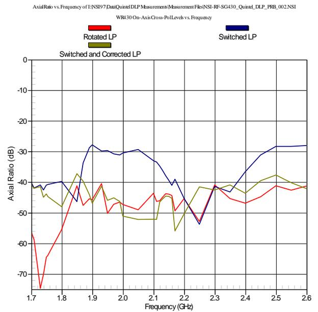
Figure 10. NSI-RF-SG430 On-Axis Cross-Pol Amplitude vs. Frequency using the Various Probe Configurations
