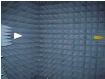
Figure 5. NSI-RF-DLP-04 Dual-Log Periodic Probe Mounted as AUT in NSI’s In-House SNF Antenna Test Facility
