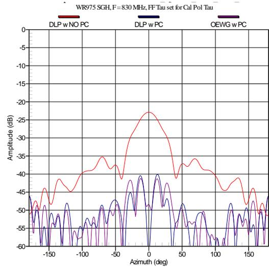
Figure 7. WR975 Standard Gain Horn E-Plane Cross-Polarization using the OEWG and DLP Probes with and without Probe Correction
