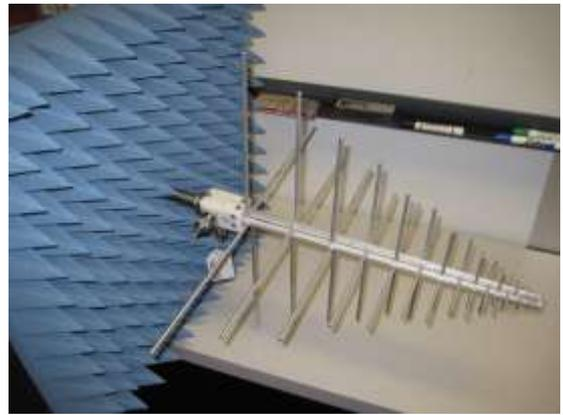
Figure 3. 300 MHz – 3 GHz Dual-Polarized Broad Band Log Periodic Probe Calibrated using this Procedure.
