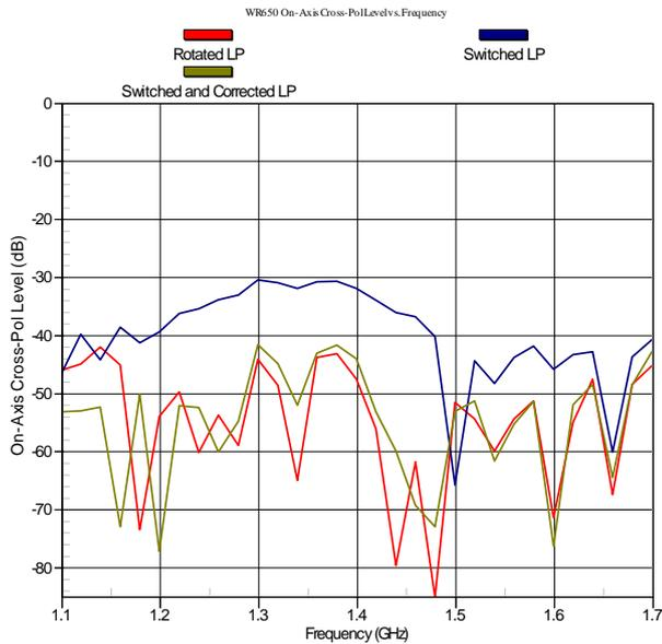
Figure 9. NSI-RF-SG650 On-Axis Cross-Pol Amplitude vs. Frequency using the Various Probe Configurations
