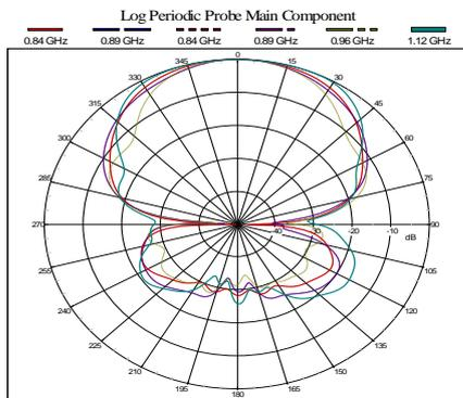
Figure 6. Log Periodic Main Component Amplitude Patterns in WR975 Band Measured During Probe Calibration Procedure
