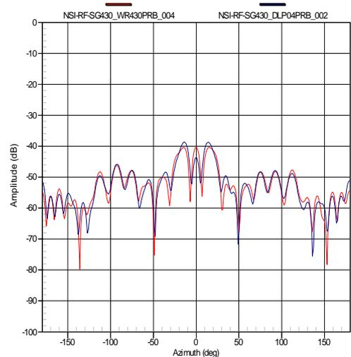
Figure 8. E-Plane Cross-Polarization Amplitude for the WR430 Standard Gain Horn Measured using the OEWG and LP Probes
