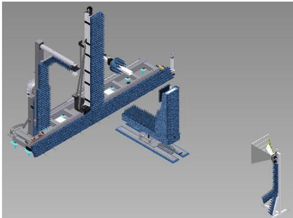
Figure 1. University of Waterloo Antenna Measurement System Layout
