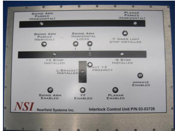
Figure 9. Front Panel Display of the Interlock Control Unit
