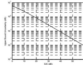
Figure 5. Amplitude measurement error due to signal-to-error ratio.
