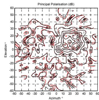
Figure 13. Contour plot comparing principal polarisations.
