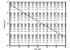
Figure 6. Phase measurement error due to signal-to-error ratio.
