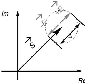
Figure 3. Worst case amplitude error,  $S$  and  $E$  in or exactly out of phase.
