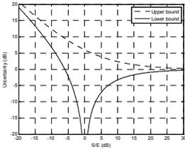
Figure 7. Upper and lower bound amplitude uncertainty plotted as a function of  $S/E$  level.
