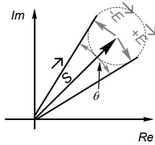
Figure 4. Worst case phase error when  $E$  and  $S + E$  are in quadrature.
