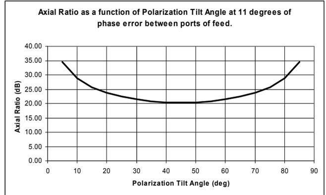
Figure 4 – Axial Ratio Sensitivity to Tilt Angle
