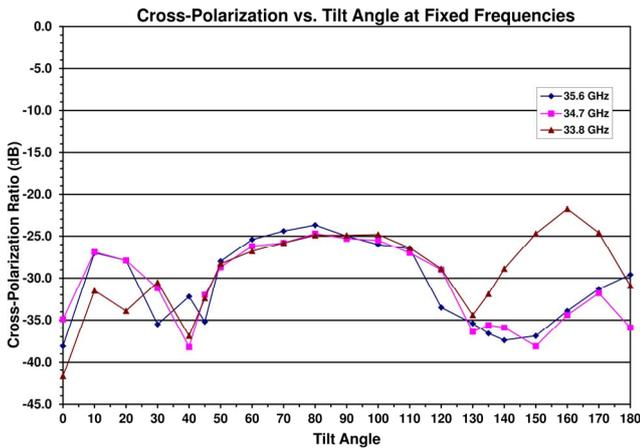
Figure 8 – Cross-polarization Performance
