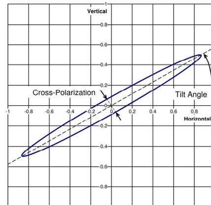
Figure 1 – Polarization Ellipse
