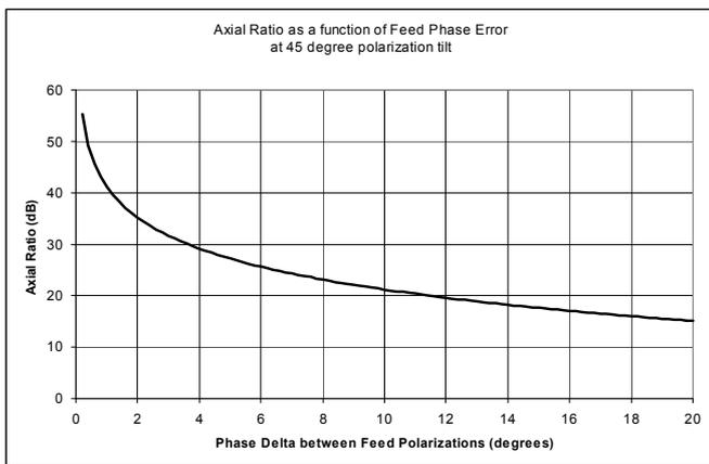
Figure 3 – Effect of Phase on Axial Ratio
