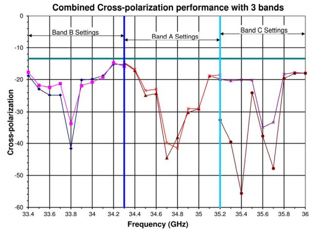
Figure 9 – Cross-polarization Bandwidth
