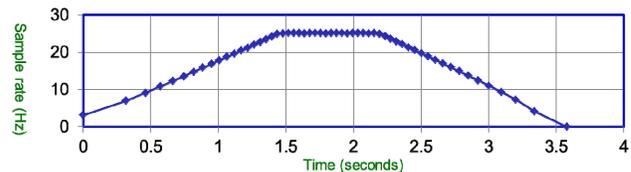
**Figure 7 – This plot shows the scan velocity during a single cut as derived from TSCI metadata.**
