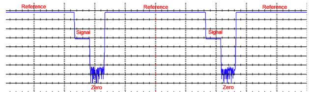
**Figure 6 – This plot shows an encoded TSCI signal magnitude waveform consisting of two antenna path transmission measurements along with the associated phase reference and zero signals. Vertical scale is 10 dB / division. Horizontal scale is 10 msec / division.**
