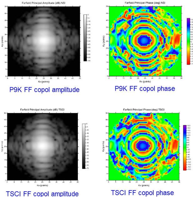
**Figure 4 – These far-field images are transformed planar near-field measurements of a 10 GHz horn antenna. The data on the top row was acquired with a standard NSI Panther 9000 receiver. The bottom row data was acquired simultaneously using the single input streaming SDR receiver. The TSCI encoding method is shown in figure 3.**
