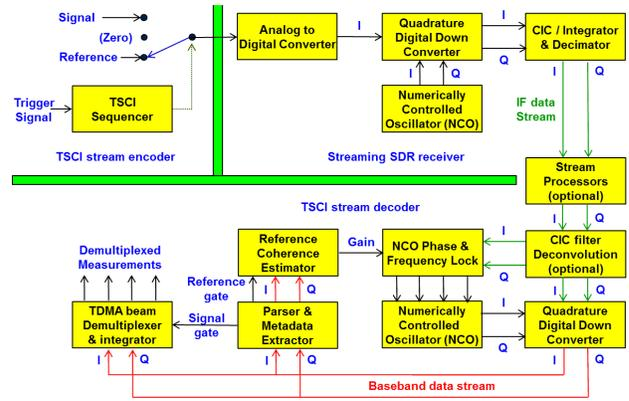
**Figure 5 – TSCI stream data flow when using a typical IF input SDR receiver or vector signal analyzer.**
