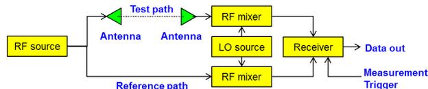
**Figure 1 - A conventional two arm interferometer directly computes the complex S21 transmission ratio between a test path and a reference path.**
