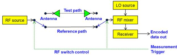
**Figure 2 - This two-arm TSCI interferometer switches between a test path and a reference path. Temporal coherence is used to infer the reference path phase when the antenna test path is selected.**
