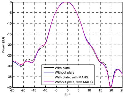
Fig 8 – Comparison of cardinal elevation cuts showing refined C-MARS processing successfully suppressing scattering in the elevation plane.
