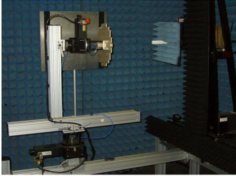
Fig 1 – NSI-200V-3x3 PCS System measuring slotted array antenna in the presence of a reflecting plate.
