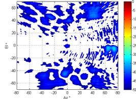
Fig. 2 – Cross-polar pattern of AUT without C-MARS processing.
