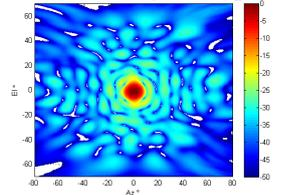
Fig. 7 – Copolar pattern of AUT with dual axis C-MARS processing.
