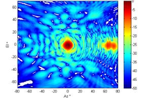
Fig. 3 – Copolar pattern of AUT without C-MARS processing.
