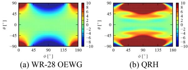
**Figure 6 – Mid-band phase patterns (units – deg)**
