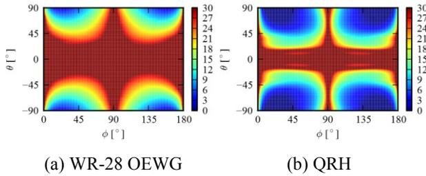
**Figure 5 – Mid-band cross-polarization discrimination (XPD) patterns (units – dB)**
