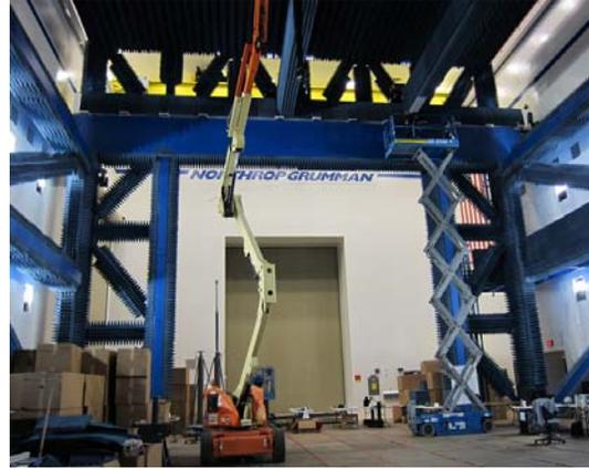
Figure 4 - NGAS Dual Bridge Near Field Scanner
