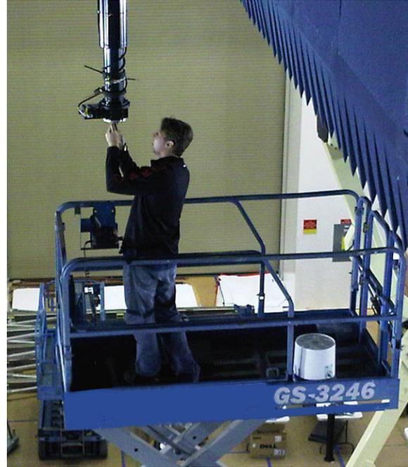
Figure 2 - Mounting of Probe Using Extension Tubes
