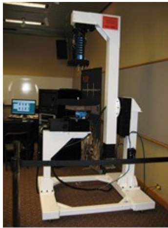
Prototype theta/phi spherical near-field test system with integrated mm-wave hardware.
