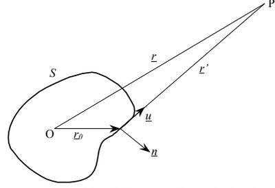
Fig. 1: Geometry of Kirchhoff-Huygens formula for the propagation of electromagnetic fields from Huygens' surface  $S$ , to point  $P$ .
