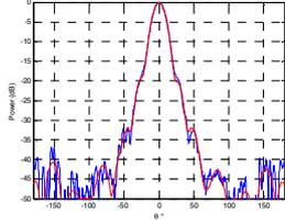
Fig.8 Amplitude with, (red) and without, (blue) F-MARS: taken without plate located at origin.
