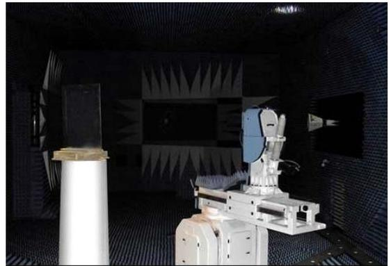
Fig. 7 Picture looking downrange in the CATR showing the AUT on the positioner and the flat rectangular scatterer placed on a low RCS polystyrene column to increase the scattering in the chamber (shown to left).
