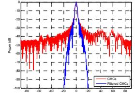
Fig. 6 Equivalent CMCs with  $\cos^2$  window applied.
