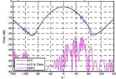
Fig. 2 Plot of the far-field pattern of the AUT with and without the reflecting plate. The specular reflection from the AUT evident in pattern & EMPL plots.
