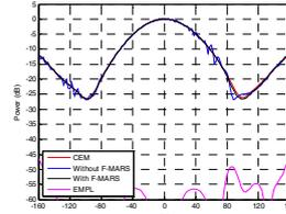
Fig. 5 Far-field pattern of AUT with ringing effectively suppressed.
