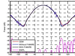
Fig. 3 Far-field pattern of AUT showing ringing from Dirichlet filter
