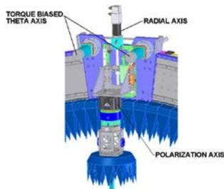
**Figure 8 – Spherical Arch Scanner Detail View**
