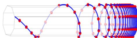
**Figure 3 – Helicoidal Scan with virtual path triggering**
