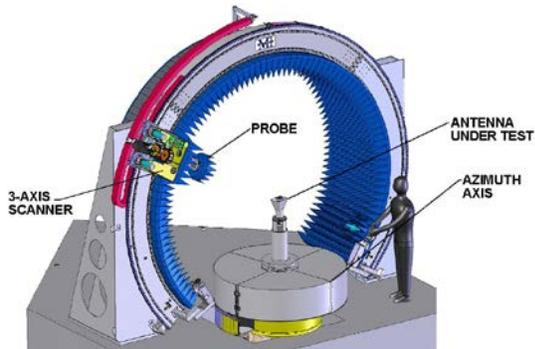
**Figure 7 –Example Spherical Arch Scanner**
