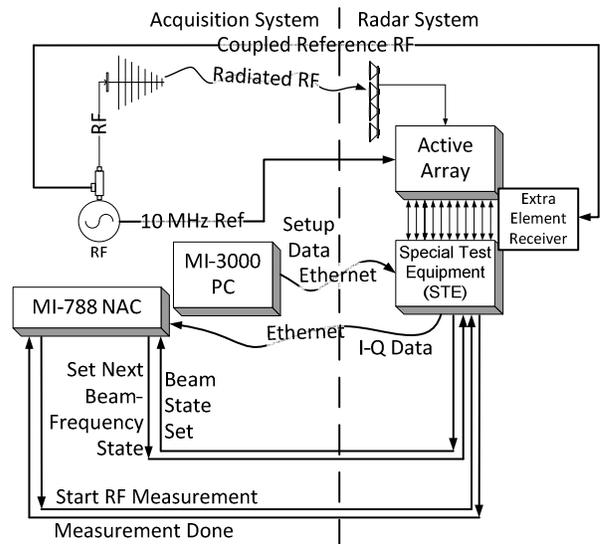
**Figure 4 – Hybrid Receive Block Diagram**
