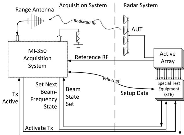
**Figure 3 – Hybrid Transmit Block Diagram**
