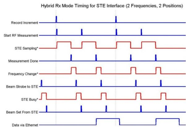
**Figure 5 – Hybrid Receive Timing Diagram**
