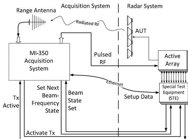
Figure 1 – Conventional Transmit Block Diagram
