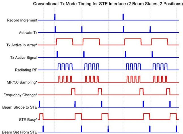
**Figure 2 – Conventional Transmit Timing Diagram**
