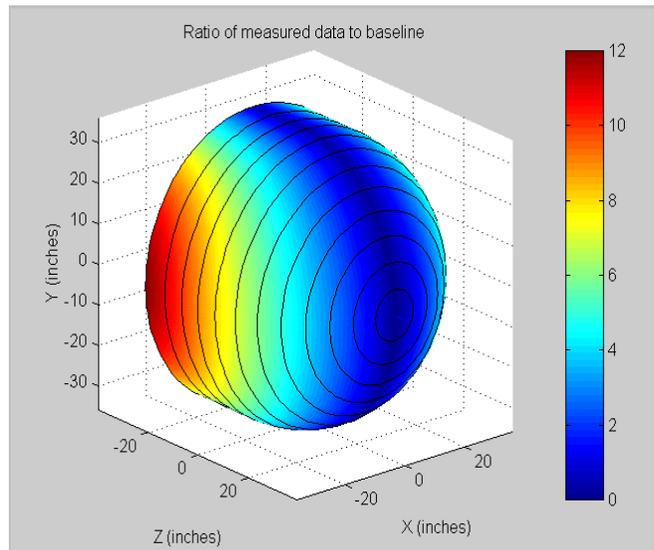
**Figure 4** Radome Test Results Plotted over Radome Surface
