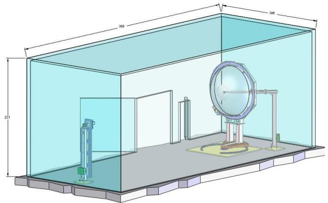
Figure 1 Radome Test Range Design
