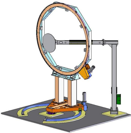
**Figure 2** Radome and System Antenna Positioner
