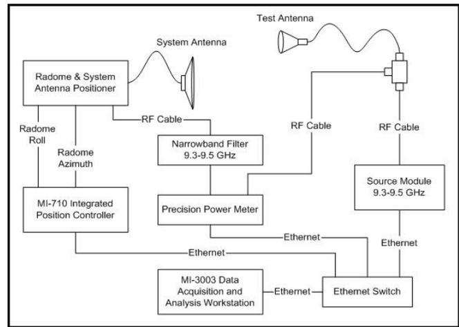
**Figure 3** Control and Instrumentation Diagram
