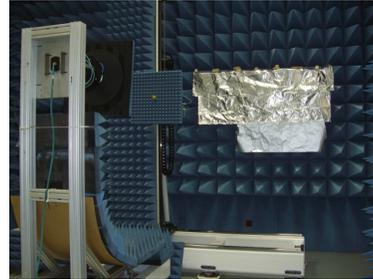
Figure 7 – NSI-300V-12x12 system shown with reflector placed behind near-field measurement scan plane measuring x-band SGH
