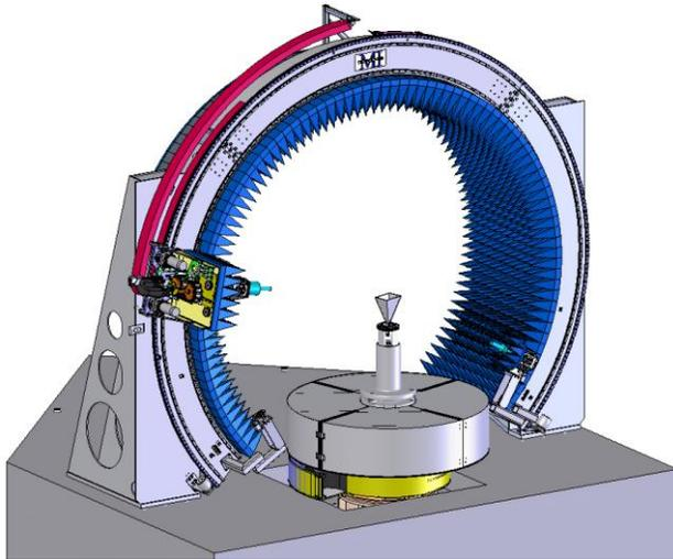
Figure 1 – SNF Measurement System
