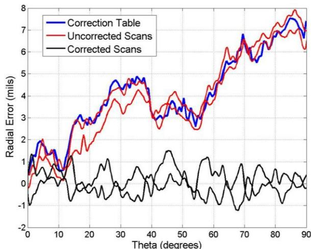
**Figure 7 – Residual Radial Errors Before and After Position Correction**
