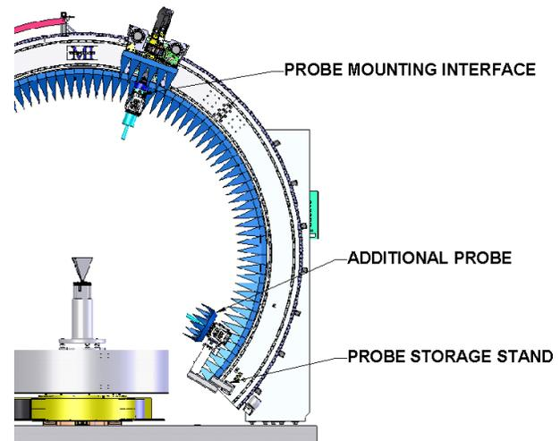
Figure 5 – Probe Changer Detail View
