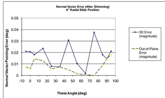
Figure 6b – Normal Vector Pointing Error After Shimming
