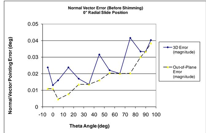
Figure 6a – Normal Vector Pointing Error Before Shimming
