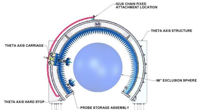
Figure 4 – Side View of Measurement System Showing Measurement Sphere
