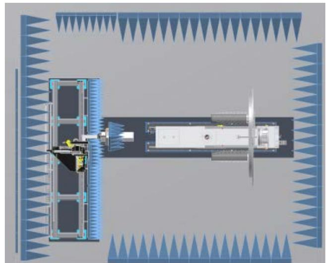
Figure 1 Spherical near-field chamber.
