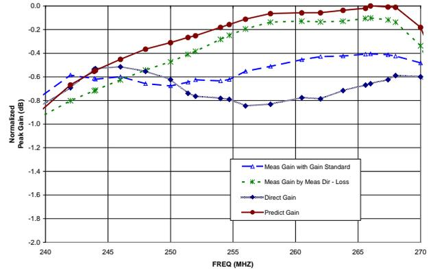
**Figure 8 Gain variation results for three measurement methods compared to predicted gain.**
