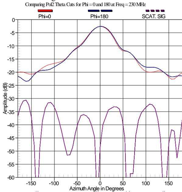
**Figure 11 Estimating room scattering for near-field data on helix gain standard.**
