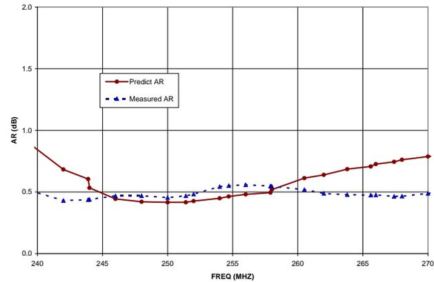
**Figure 9 Axial ratio results compared to predicted values.**
