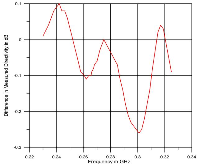
**Figure 7 Directivity difference of gain standard from measurements with and without probe absorber.**
