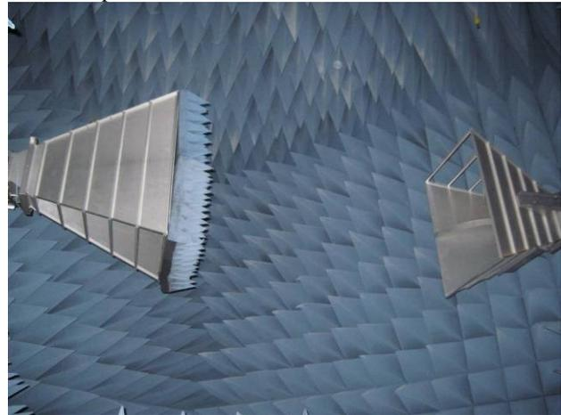
Figure 5 Two dual ridged horns in the spherical chamber during the probe pattern measurements.
