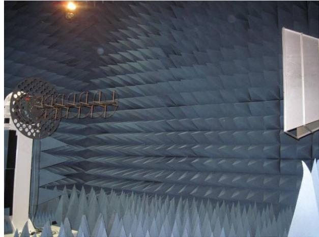
Figure 4 Single element helix gain standard in the spherical near-field chamber with the horn probe.
