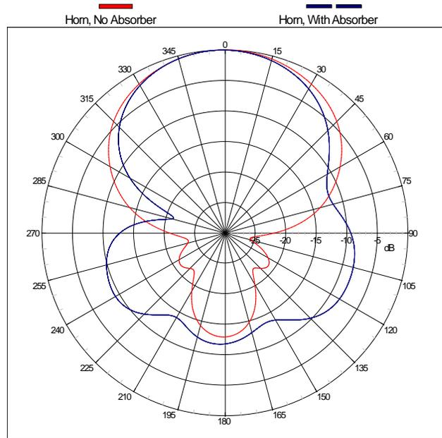
**Figure 6 Horn probe far-field patterns with and without the absorber panel at 230 MHz.**
