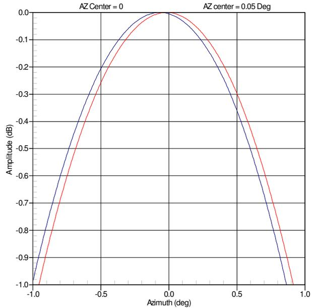
Figure 2 Expanded main beam plots used to estimate beam offset errors.
