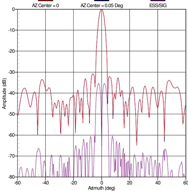
Figure 1 Simulated pattern comparison where the second pattern is identical to the first but shifted by 0.05 degrees.
