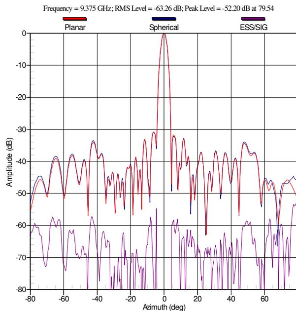
**Figure 5 Example of pattern comparison between a planar and spherical near-field range.**
