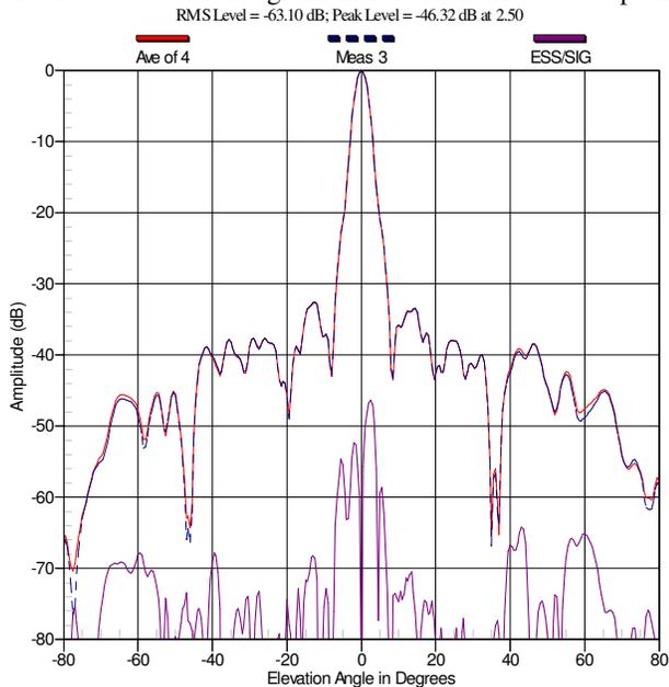
**Figure 3 Comparing the far-fields computed from the average of four measurements at different z-distances with a single result to estimate multiple reflection uncertainty.**
