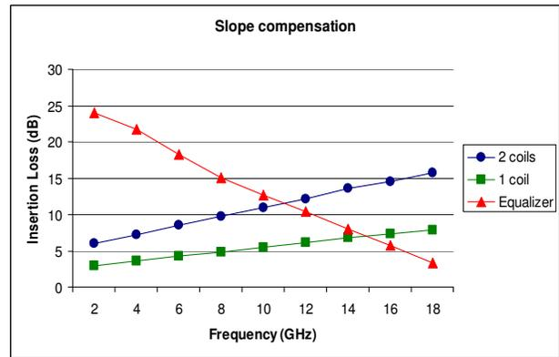
**Figure 4 Slope compensation using positive slope equalization coils with a negative slope equalizer**
