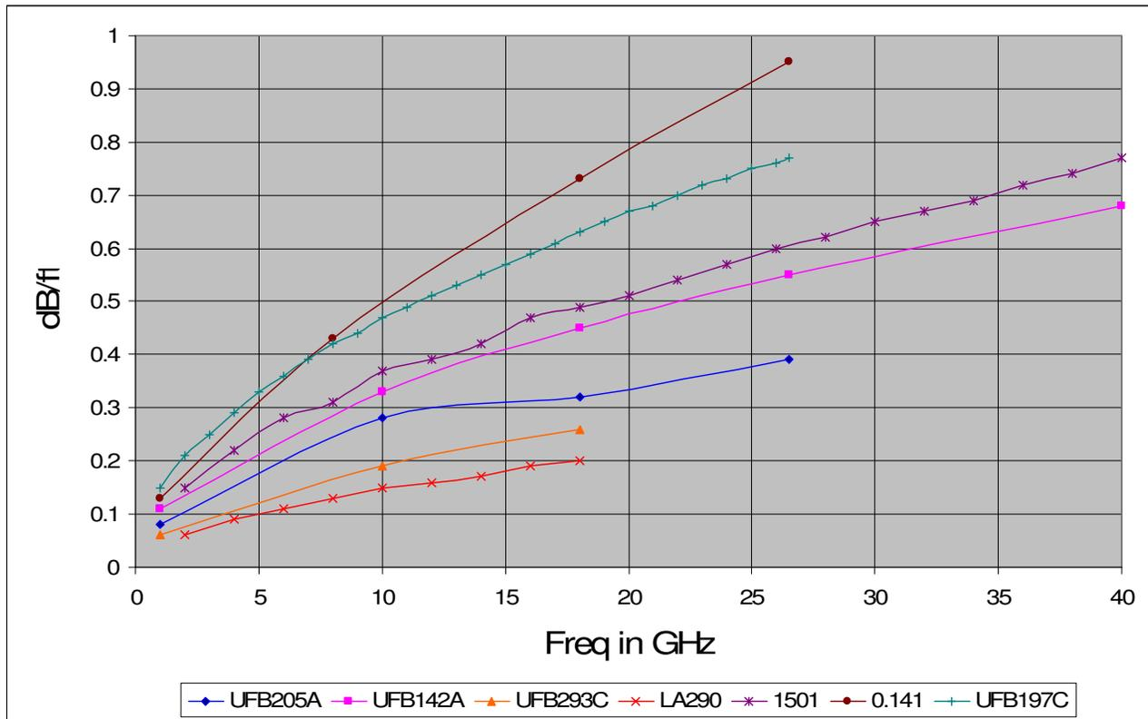
Figure 3 – Insertion loss specifications for typical low loss RF coaxial cables
