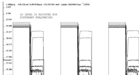
**Figure 6: The software adjusts the attenuation values across different frequencies**
