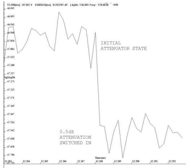
**Figure 5: Attenuator switching speed**
