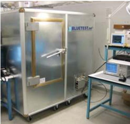
**Figure 2** Typical reverberation chamber.
