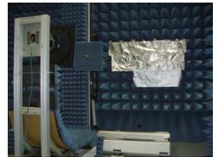
Figure 15 – NSI-300V-12x12 shown with reflector placed behind scan plane
