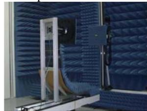
Figure 14 – NSI-300V-12x12 system installed within a partially absorber lined chamber
