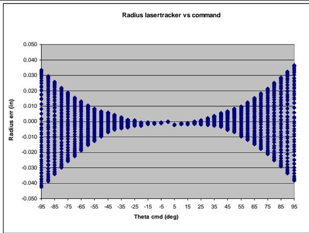
**Figure 10 – Laser tracker measurements of uncorrected Radius error over  $\pm 95^\circ$  Theta for all Phi angles**
