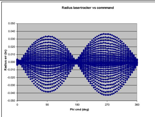
**Figure 11 – Laser tracker measurements of uncorrected Radius error over  $360^\circ$  Phi for all Theta angles**
