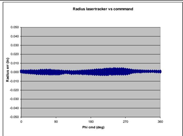
**Figure 13 – Laser tracker measurements of corrected Radius error over  $360^\circ$  Phi for all Theta angles**
