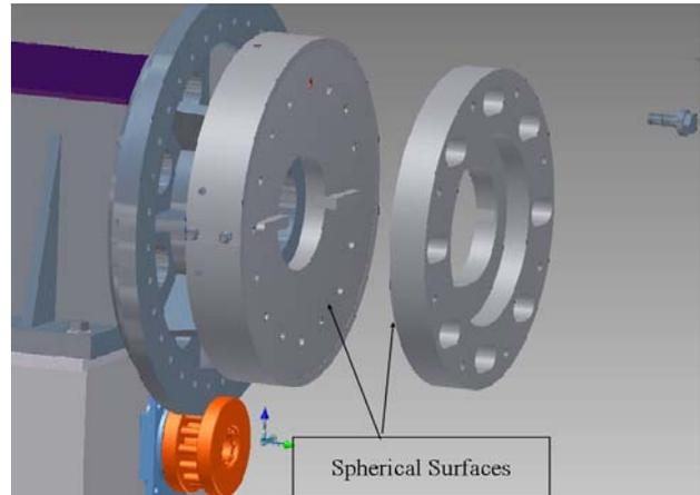
**Figure 5 – Spherical adjustment fixture for mounting and aligning Theta structure to Phi stage**
