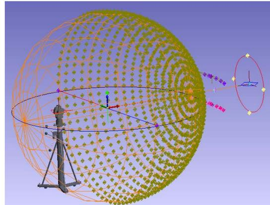
**Figure 9 – Laser tracker measurements over  $360^\circ$  Phi and  $\pm 90^\circ$  Theta**
