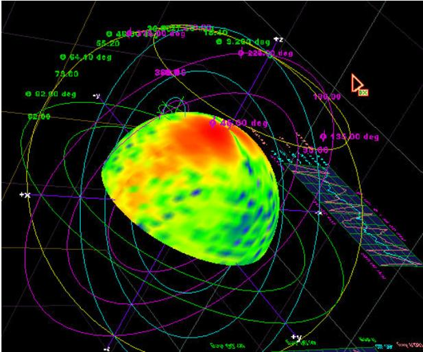
**Figure 2 - Typical hyper-hemispherical near-field data measured on NSI-700S-300**
