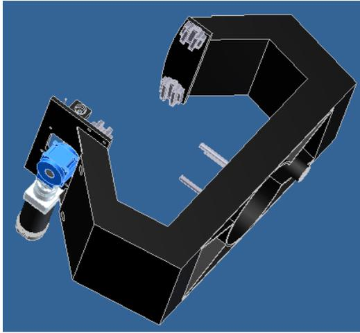
**Figure 7 – Theta Carriage for Probe Motion**
