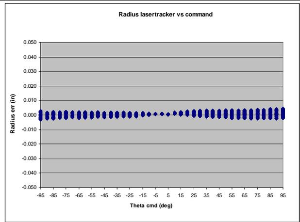
**Figure 12 – Laser tracker measurements of corrected Radius error over  $\pm 95^\circ$  Theta for all Phi angles**
