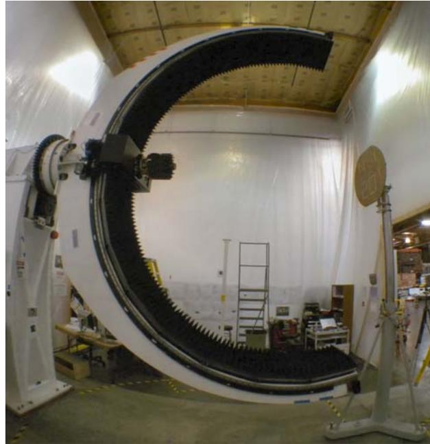
**Figure 3 - NSI-700S-300 arch roll spherical scanner during factory testing**
