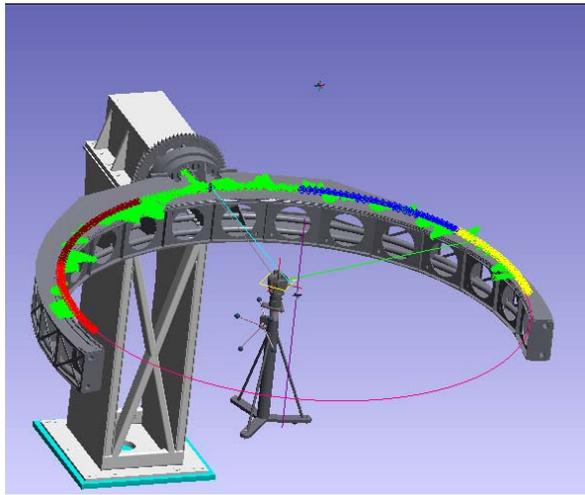
**Figure 8 – Laser tracker metrology during system assembly & alignment**
