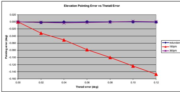
**Figure 9– WR28 WG Array Elevation beam pointing error vs Theta-zero error for different SNF measurement geometries**
