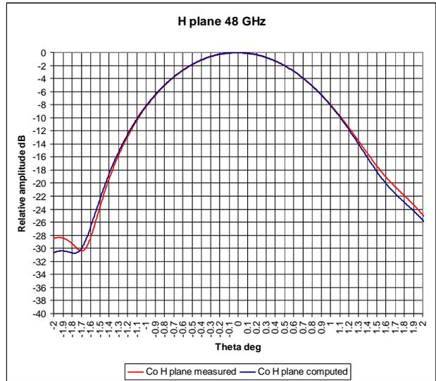
Figure 15- QVCA H plane measured and computed patterns
