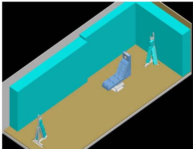
**Figure 5– NSI-700S-60 Spherical Near-field / Far-field**
