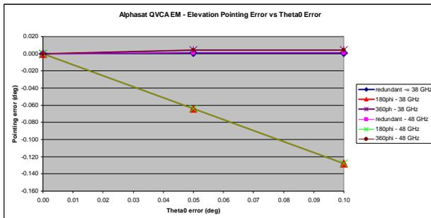
**Figure 10– Alphasat QVCA EM Elevation beam pointing error vs Theta-zero error for different SNF measurement geometries**
