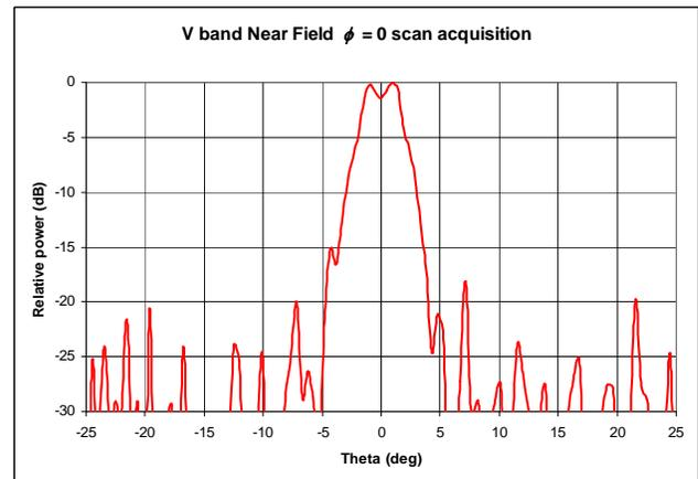
**Figure 12- QVCA EM scan window (including practically all the antenna energy)**
