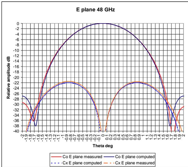
Figure 14- QVCA E plane measured and computed patterns
