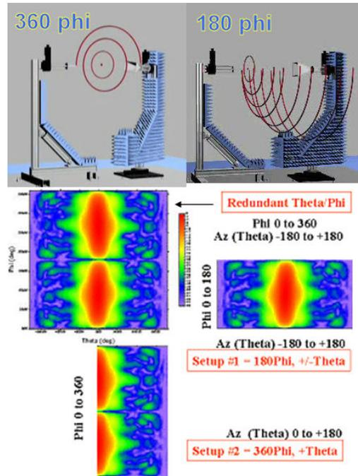
Figure 7– Redundant data set through full rotation of theta and phi rotators, versus the two full spheres that can be derived for the “360 phi” or “180 phi” configurations
