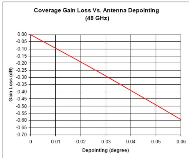
Figure 16– QVCA link losses Vs. beam misalignment
