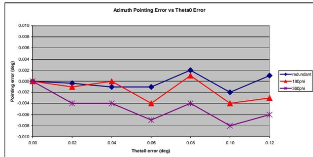
Figure 8– WR28 WG Array Azimuth beam pointing error vs Theta-zero error for different SNF measurement geometries
