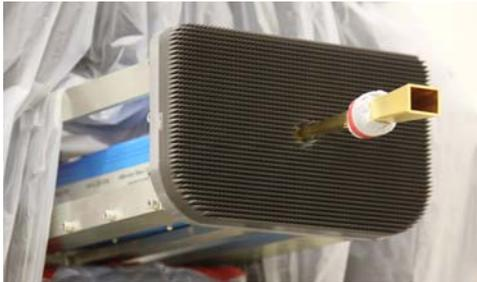
**Figure 3** Photo of Zax carbon loaded dielectric absorber behind 140-220 GHz horn
