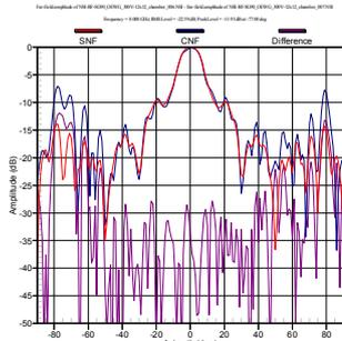
Fig. 14 Azimuth cuts from Spherical and cylindrical at 8.0 GHz without MARS processing
