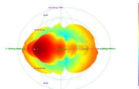
Fig. 10 Far-field pattern obtained from spherical measurement
