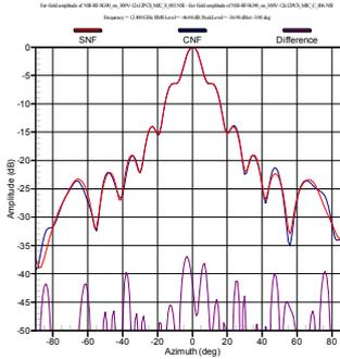
Fig. 17 Spherical and cylindrical azimuth cuts at 12.4 GHz with MARS processing
