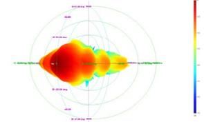
Fig. 13 Far-field pattern obtained from cylindrical measurement with cylindrical MARS processing
