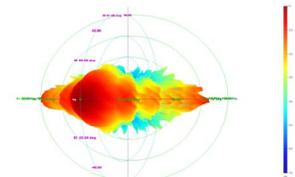
Fig. 11 Far-field pattern obtained from cylindrical measurement
