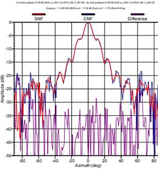
Fig. 16 Spherical and cylindrical azimuth cuts at 12.4 GHz without MARS processing
