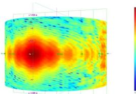
Fig. 4 Horizontally polarised measured cylindrical near-field component
