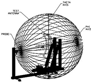
Fig. 1 Spherical positioning system and measurement geometry
