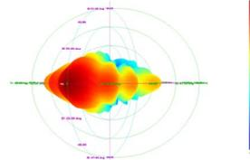
Fig. 12 Far-field pattern obtained from spherical measurement with spherical MARS processing
