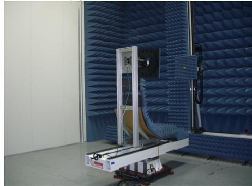
Fig. 9 NSI-300V-12x12 PCS system shown taking near-field measurements of NSI-RF-SG90 in a partially anechoic environment. Here, absorber placement has been optimised for planar acquisition mode.
